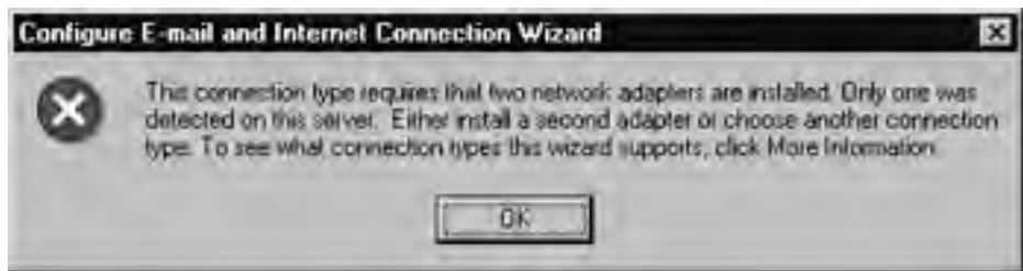
Figure 3.8 Network Interface Card Requirement Warning
