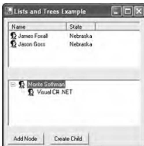
Figure 8.9. You can create as deep a hierarchy as you need using the Tree View control.
