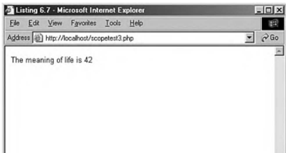
Figure 6.5. Successfully accessing a global variable from within a function using the global keyword.
