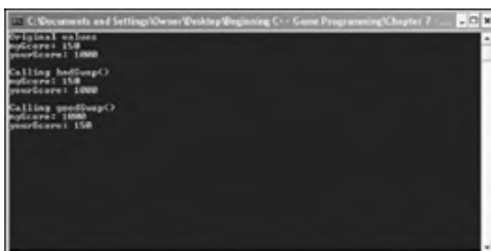
Figure 7.3: Passing pointers allows a function to alter variables outside of the function's scope.
