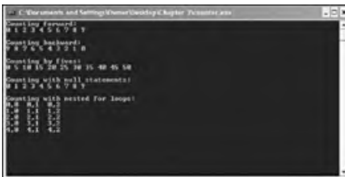
Figure 3.1: for loops do all of the counting, while a pair of nested for loops displays the grid.
