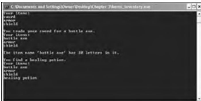
Figure 3.4: The hero's inventory is a sequence of string objects stored in an array.
