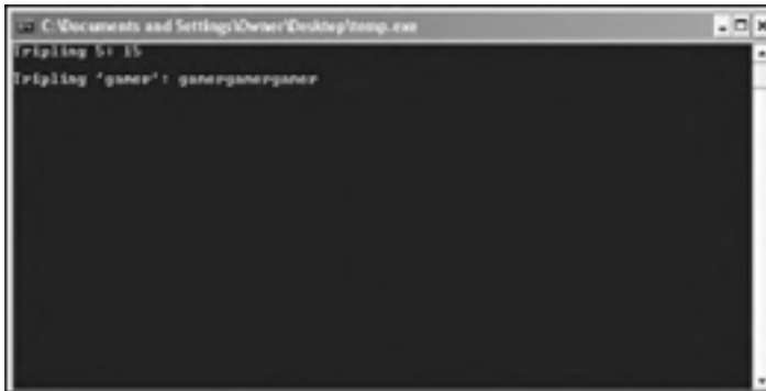
Figure 5.6: Function overloading allows you to triple the values of two different types using the same function name.
