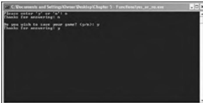
Figure 5.2: Each question is asked by a separate function, and information is passed between these functions and main() .
