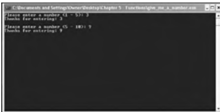
Figure 5.5: A default argument is used for the lower limit the first time the user is prompted for a number.
