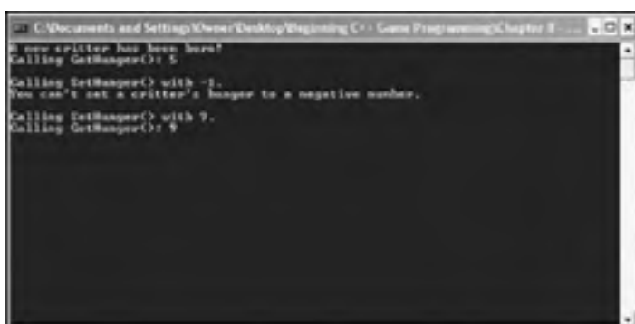
Figure 8.3: By using a Critter object's GetHunger() and SetHunger() member functions, the program indirectly accesses an object's private m_Hunger data member.
