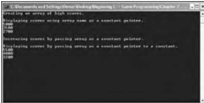
Figure 7.8: Using an array name as a pointer, the high scores are displayed, altered, and passed to functions.
