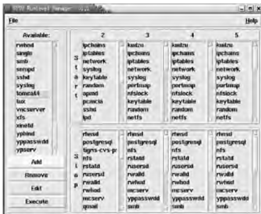
Figure 1-8. Adding the tomcat4 service in tksysv on Linux
