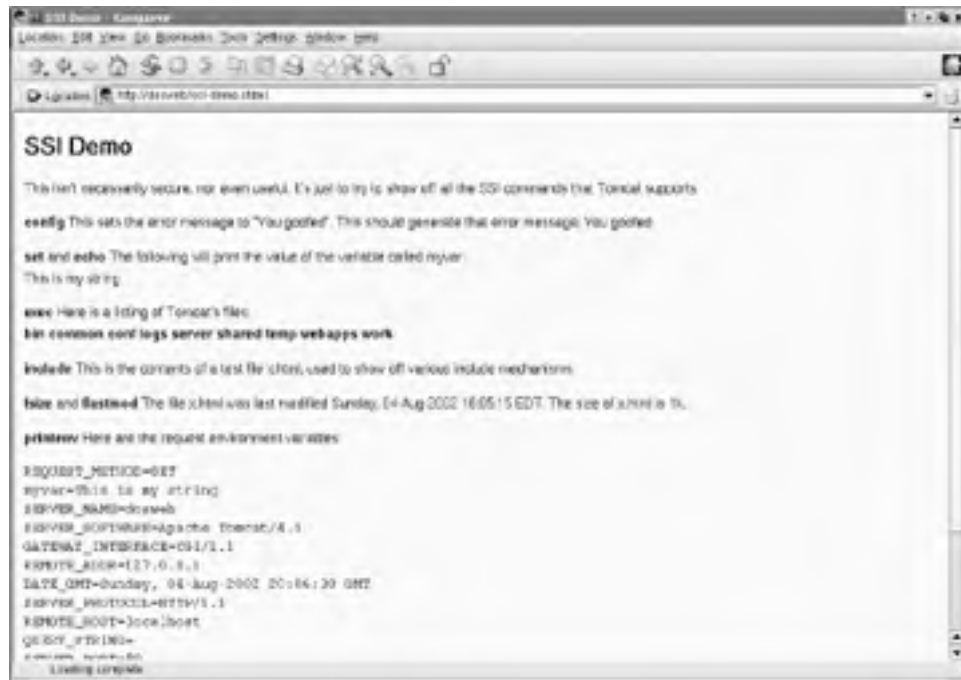
Figure 2-1. SSI output from ssi-demo.shtml
