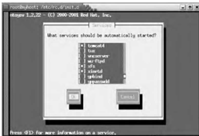
Figure 1-9. Adding the tomcat4 service in ntsysv on Linux
