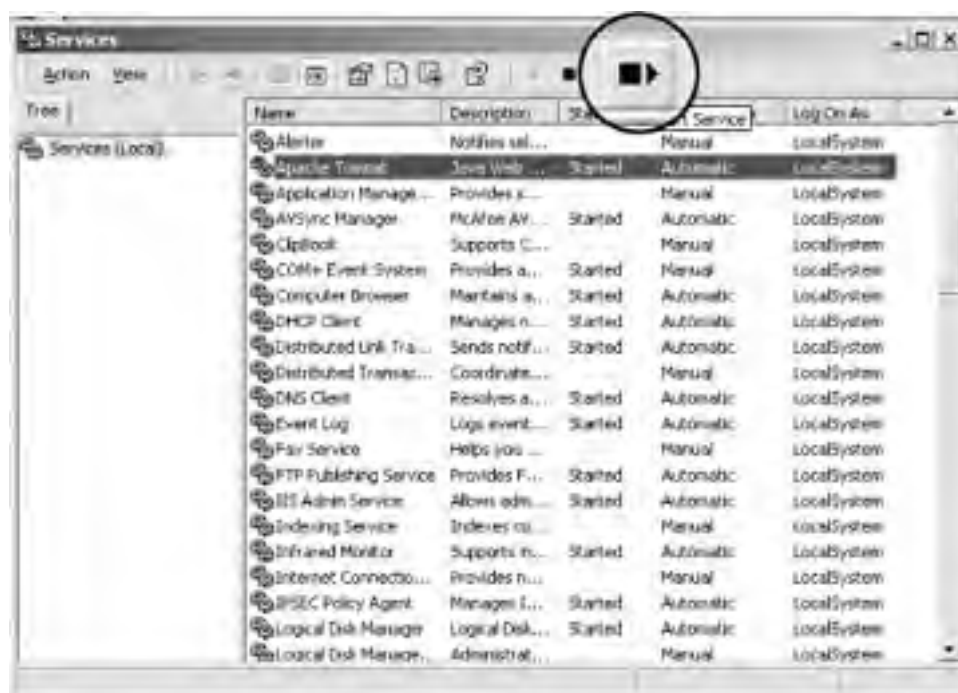
Figure 1-7. Restart button in the Control Panel
