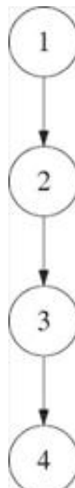
Figure 3.2. Chain of processes generated by Program 3.1 when called with a command-line argument of 4.
