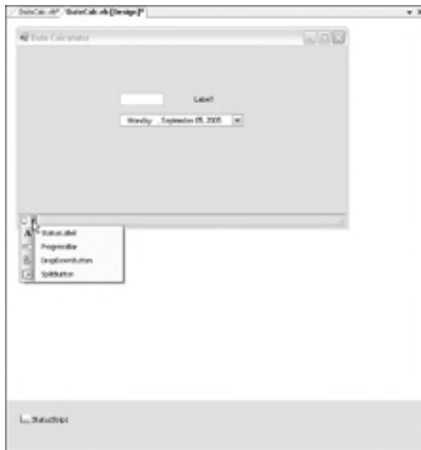
Figure 4-10: Adding a status bar to the Date Calculator.
