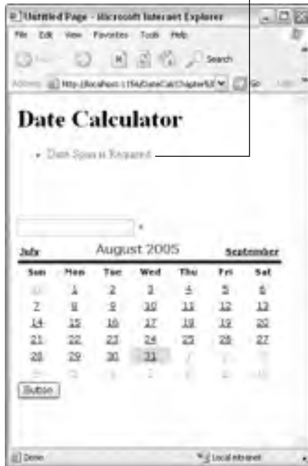
Figure 5-12: Input validation in action.
