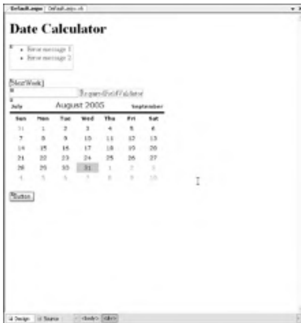
Figure 5-11: My application's Design View after putting in the text box and Validation controls.
