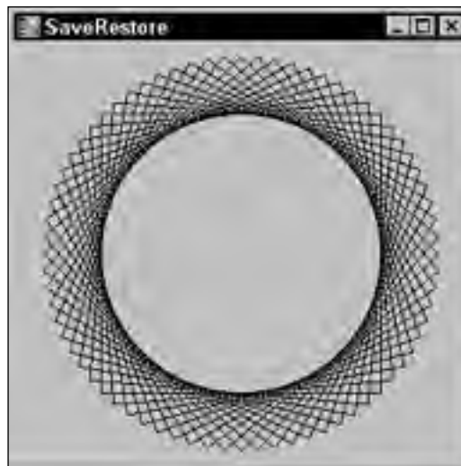
Figure 19-21: This program saves and restores the Graphics object's state containing a scaling and translation, adding an extra rotation as needed.
