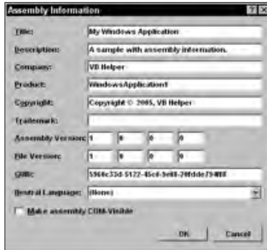
Figure 3-3: The Assembly Information dialog lets you define basic project information such as title, copyright, and version number.
