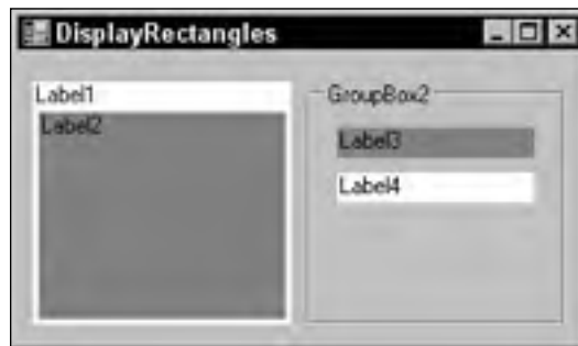
Figure A-1: The DisplayRectangle property gives the area in which you should normally place items within a control.
