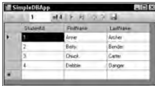
Figure 11-13: Drag and drop a table from the Data Sources window onto the form to create a simple DataGridView .
