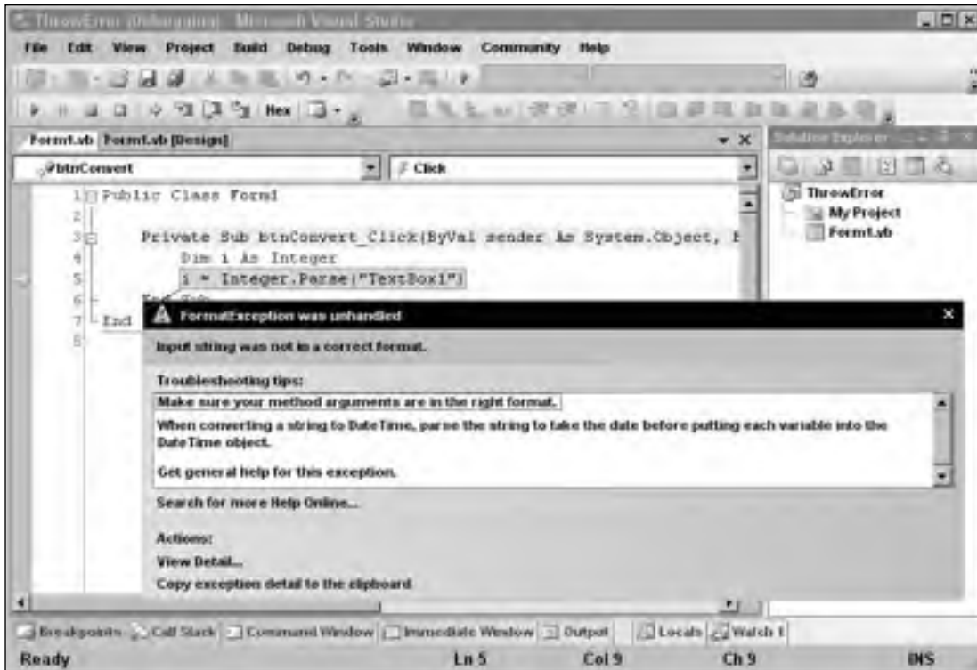
Figure 8-1: When a program crashes, the message it generates tells you the type of exception it raised.
