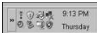
Figure 10-6: An application can use a NotifyIcon control to display status icons in the system tray.
