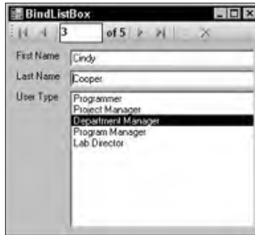
Figure 11-34: The steps for binding a ListBox are the same as those for binding a ComboBox .
