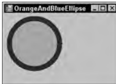
Figure 19-1: This program uses SolidBrush and Pen objects to draw an orange circle with a wide blue outline.
