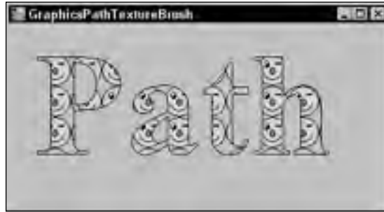
Figure 20-13: A program can use a Graphics object's FillPath and DrawPath methods to fill and draw a GraphicsPath object.
