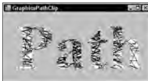
Figure 20-15: A program can use a GraphicsPath object to define a clipping region.
