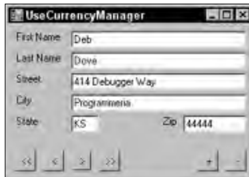
Figure 11-29: This program's buttons use a CurrencyManager to let the user add, delete, and navigate through a table's records.
