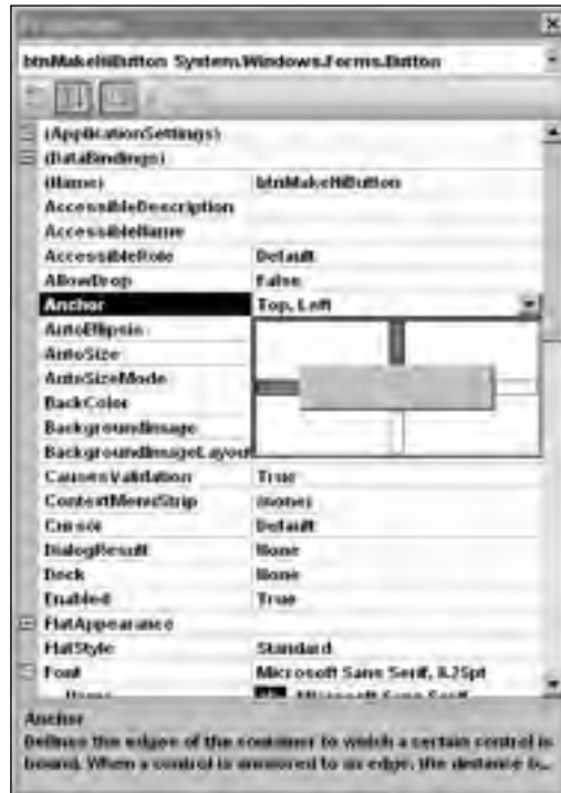
Figure 2-9: Some properties, such as Anchor , provide specialized editors to let you select their values.
