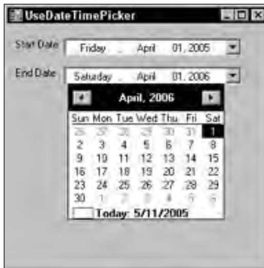
Figure G-4: The DateTimePicker control lets the user select a date and time.
