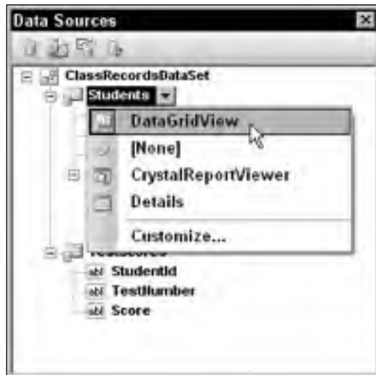
Figure 11-15: Use the drop-down in the Data Sources window to give a table a different display style.
