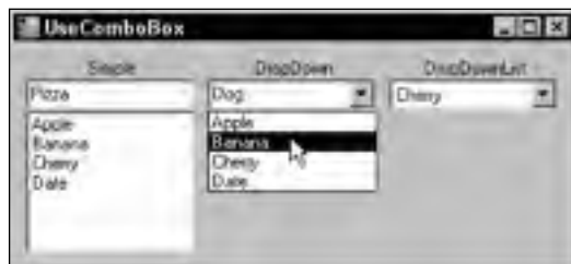
Figure G-3: The ComboBox provides three different styles: Simple , DropDown , and DropDownList .
