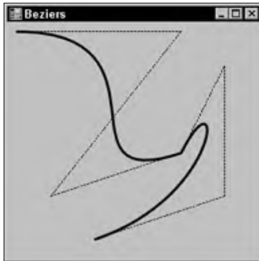
Figure 19-8: The DrawBeziers method draws a series of Bézier curves with common end points.
