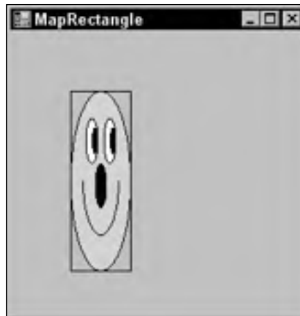
Figure 19-19: The MapRectangles subroutine can stretch a drawing by different amounts vertically and horizontally.
