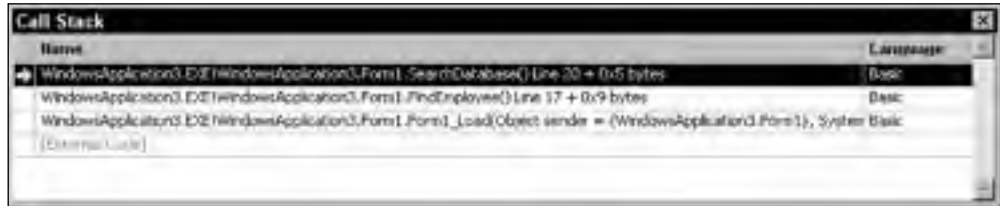
Figure 1-30: The Call Stack window shows which routines have called which to get to the program's current point of execution.
