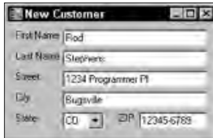
Figure 2-15: This dialog uses Anchor properties to make its TextBox controls use whatever space is available on the form.
