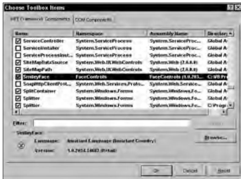
Figure 12-2: Use the Customize Toolbox dialog to add your control to the Toolbox.
