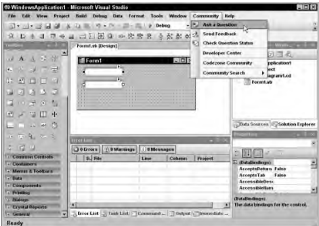
Figure 1-49: The Community menu contains commands that give access to Microsoft's Visual Basic developer community.
