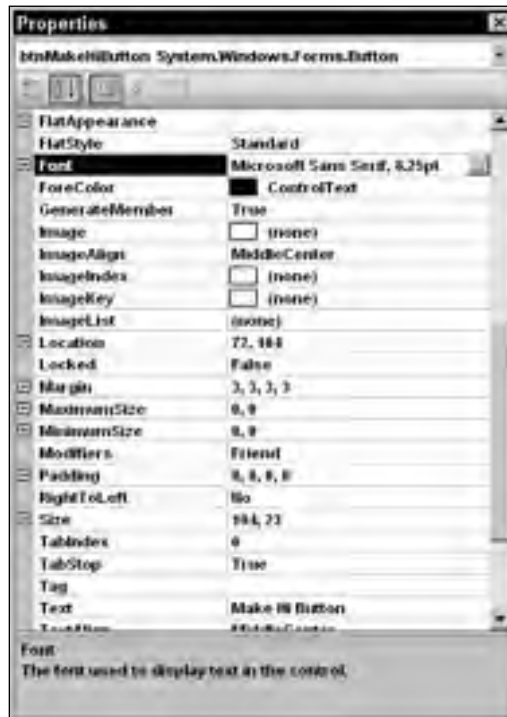
Figure 2-5: The Properties window lets you change a control's properties at design time.
