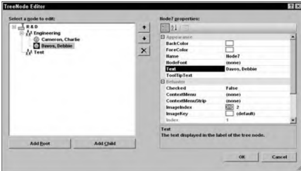
Figure G-31: The TreeNode Editor lets you edit a TreeView control's data at design time.
