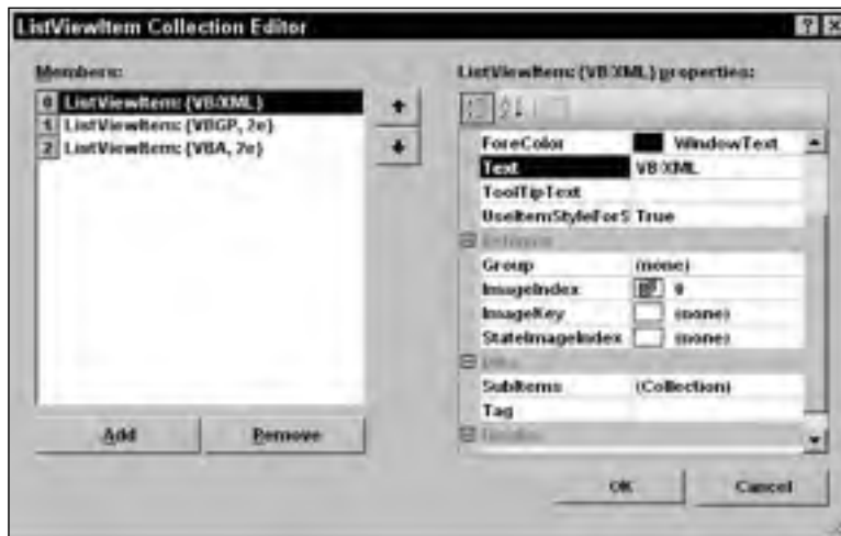
Figure G-9: Use the ListViewItem Collection Editor to define a ListView control's items at design time.
