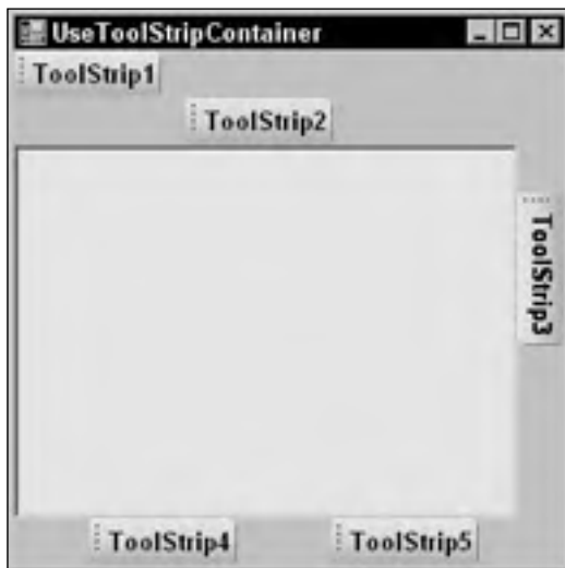
Figure G-29: The ToolStripContainer control lets the user rearranged ToolStrip controls at run time.
