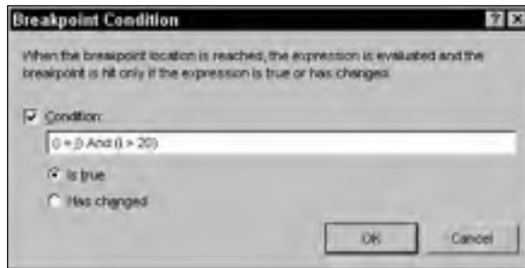
Figure 1-33: The Breakpoint Condition dialog lets you specify a condition that determines whether Visual Studio stops at the breakpoint.
