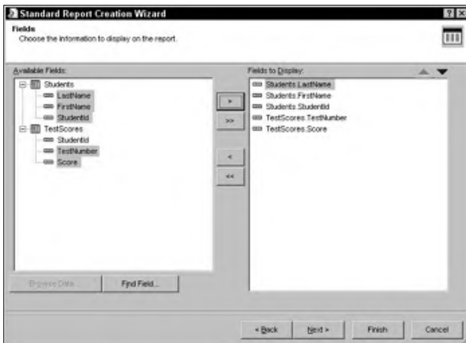
Figure 24-8: Use the Fields page to select the fields displayed by the report.
