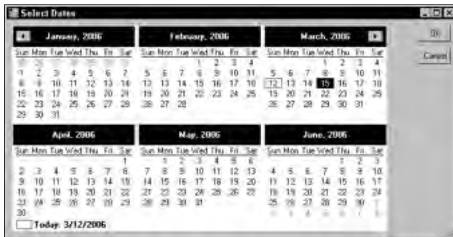
Figure G-13: The MonthCalendar control can display more than one month at a time.
