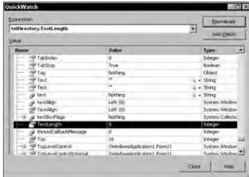
Figure 1-24: The QuickWatch dialog lets you examine an object’s properties and optionally set a new watch on it.
