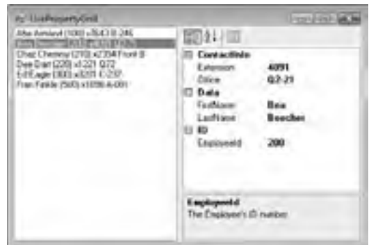
FIGURE G-8: The PropertyGrid control displays an object's properties.
