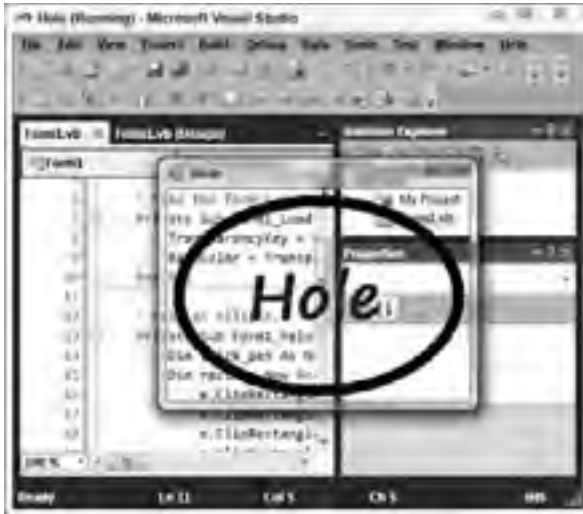
FIGURE 10-2: A form's TransparencyKey property lets you make shaped forms such as this one with a hole in it.
