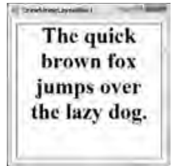
FIGURE 32-2: The DrawString method can use a layout rectangle and a StringFormat object to format text.
