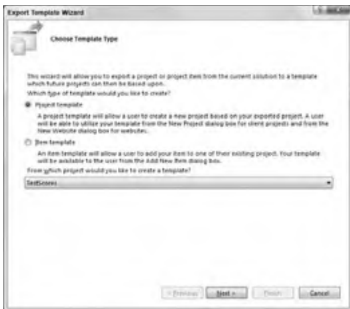
FIGURE 2-3: The File/Export Template command displays this dialog box to help you create project or items templates that you can easily use in other projects.
