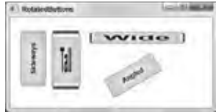
FIGURE 12-6: Buttons can be rotated and scaled vertically and horizontally by using RotateTransform and ScaleTransform .
