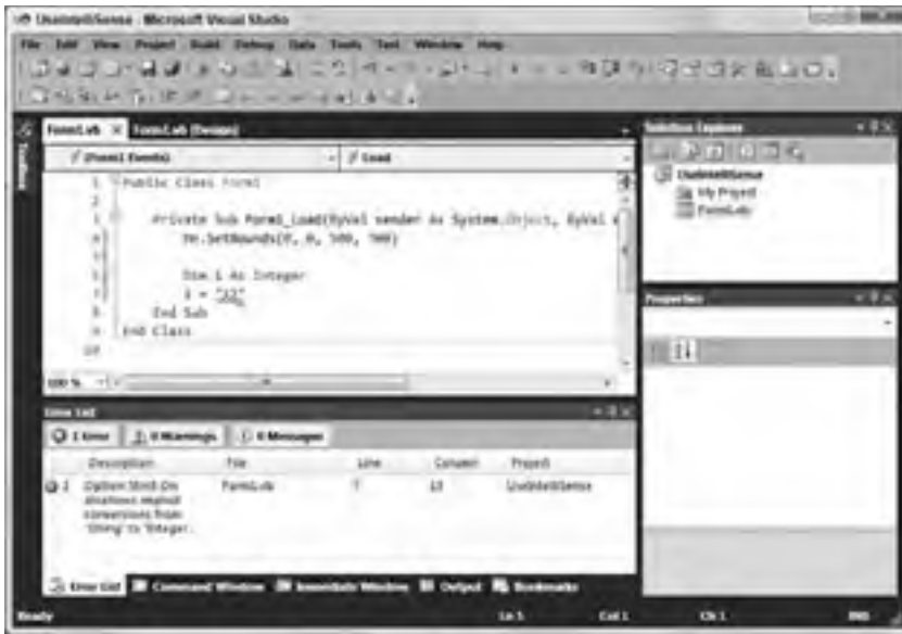
FIGURE 6-6: If the code editor thinks it can figure out what's wrong, it displays a suggestion indicator.
