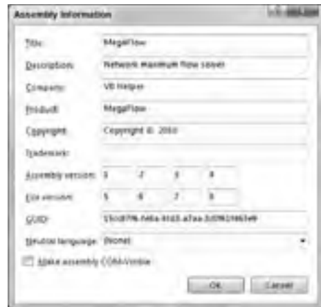
FIGURE S-1: Use this dialog box to enter information that the program can later retrieve using My.Application.AssemblyInfo.
