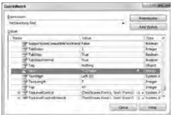
FIGURE 7-1: The QuickWatch dialog box lets you examine an object's properties and optionally set a new watch on it.
