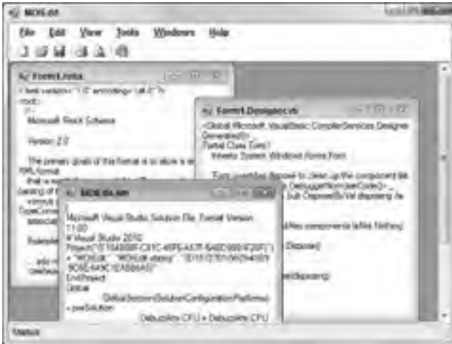
FIGURE 10-7: An MDI application displays documents in forms contained within an MDI container form.
