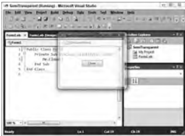
FIGURE 10-1: A form with Opacity set to 66% allows the Visual Basic IDE to show through.
