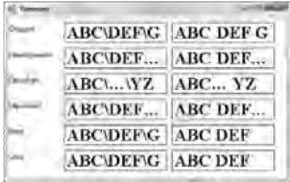
FIGURE 32-7: The StringFormat object's Trimming property determines how text is trimmed.
