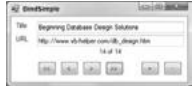
FIGURE 20-21: This program's buttons use a CurrencyManager to let the user add, delete, and navigate through a table's records.
