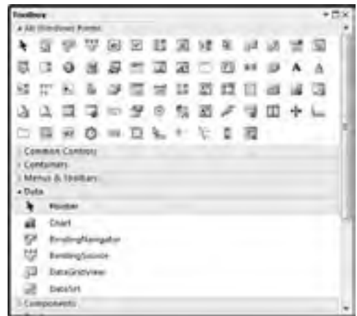
FIGURE 2-13: The Toolbox window can display tools by name or icon.
