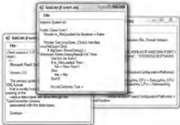
FIGURE 10-6: An SDI application displays separate documents in separate forms.
