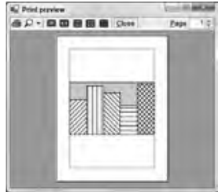
FIGURE 34-6: Subroutine FitPictureToMargins makes it easy to center a picture within a printed page, making it as large as possible without distortion.
