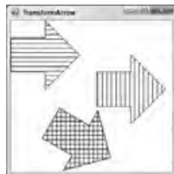
FIGURE 30-10: This program draws arrows scaled, translated, and rotated.
