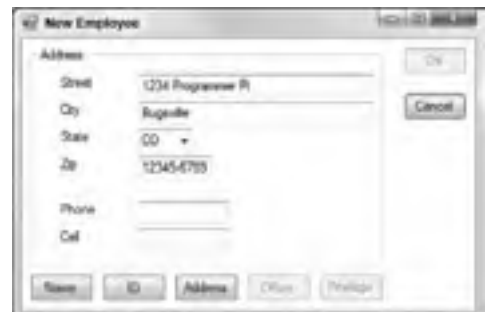
FIGURE 10-11: This wizard uses buttons instead of tabs to move through its pages of data.
