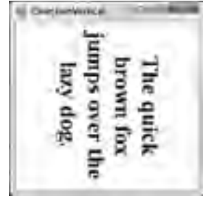
FIGURE 32-4: Setting the StringFormat object’s FormatFlags property to DirectionVertical produces vertical text.
