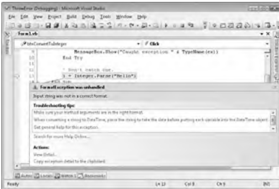
FIGURE 19-1: When a program crashes, the message it generates tells you the type of exception it raised.
