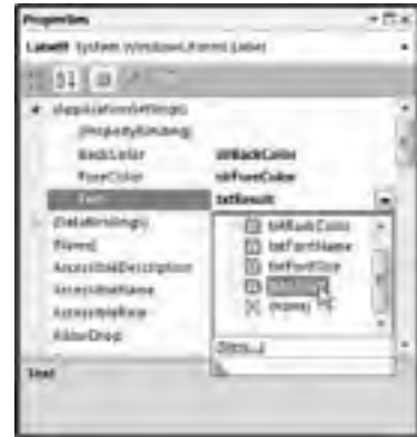
FIGURE 35-2: Use the drop-down list to assign a setting to the dynamic property.
