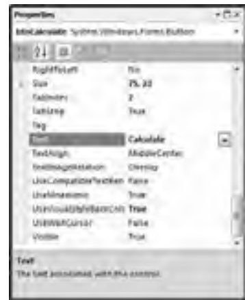
FIGURE 2-15: The Properties window lets you view and modify control properties.
