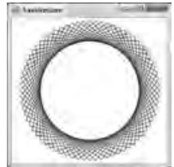
FIGURE 30-12: This program saves and restores the Graphics object's state containing a scaling and translation, adding an extra rotation as needed.
