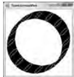
FIGURE 31-5: The white ellipses show where the Pen object's transformed tip was as it drew the large black circle.
