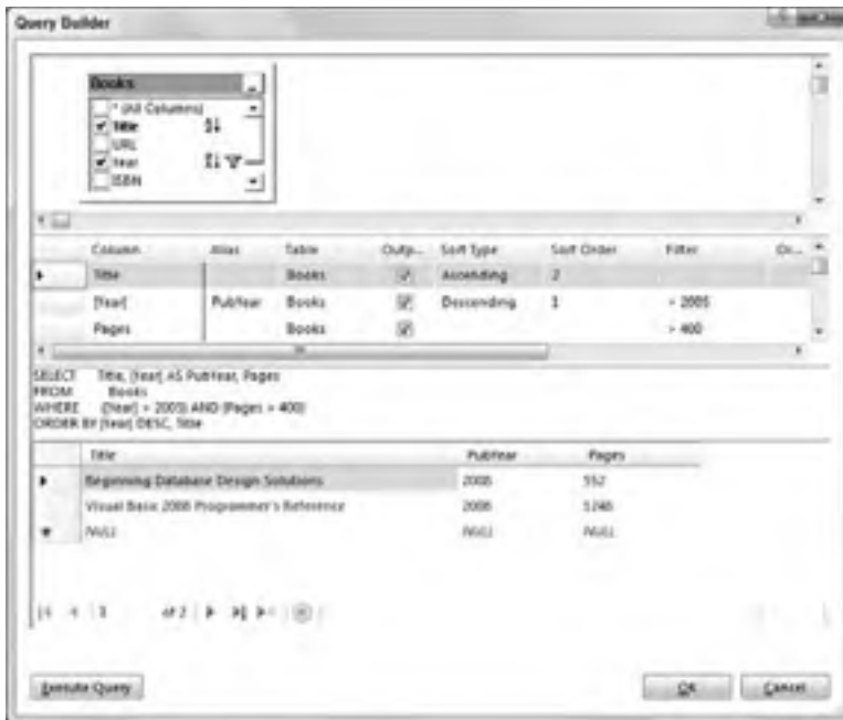
FIGURE 20-17: You can use the Query Builder to interactively define the data that a data adapter selects.
