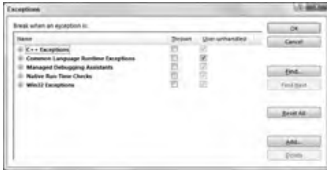
FIGURE 7-3: The Exceptions dialog box lets you determine how Visual Basic handles uncaught exceptions.
