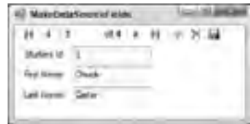
FIGURE 20-11: Drag and drop table columns onto a form to create a record-oriented view instead of a grid.
