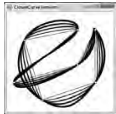
FIGURE 30-8: The DrawClosedCurve method's tension parameter determines how tightly the curve bends.
