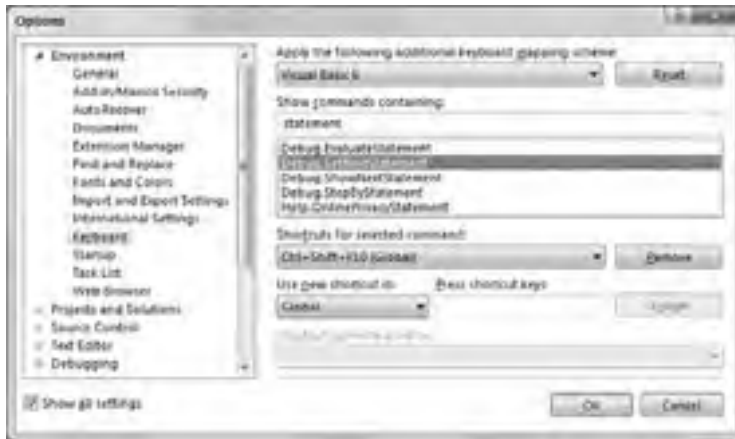
FIGURE 3-3: The Options dialog’s Keyboard section lets you view and modify keyboard shortcuts.
