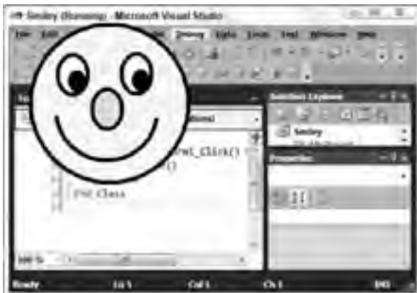
FIGURE 10-3: The TransparencyKey property lets you make shaped forms such as this one.
