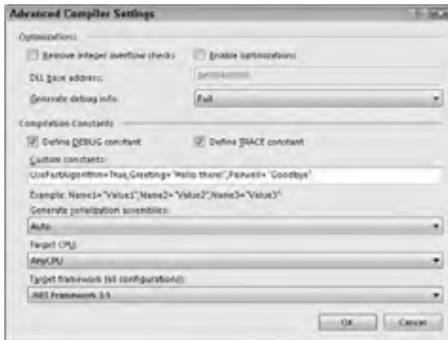
FIGURE 14-4: Use the Advanced Compiler Settings dialog box to define compilation constants.
