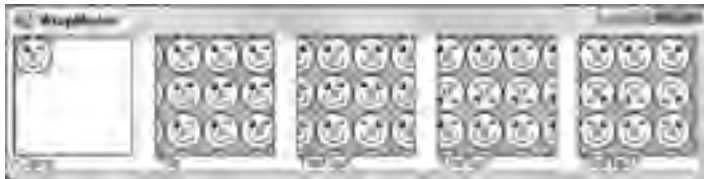
FIGURE 31-6: The TextureBrush class's WrapMode property determines how the brush tiles its image.
