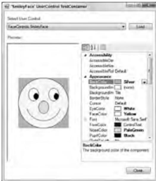
FIGURE 22-1: Visual Basic lets you preview controls in the UserControl Test Container.
