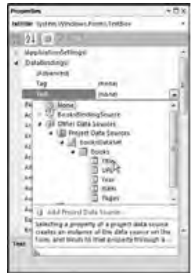
FIGURE 20-20: You can bind a simple control property to a data source at design time.
