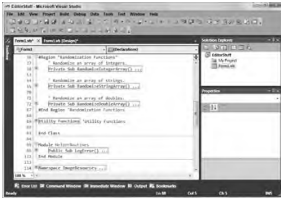
FIGURE 6-2: The code editor outlines namespaces, classes and their methods, modules and their methods, and regions.
