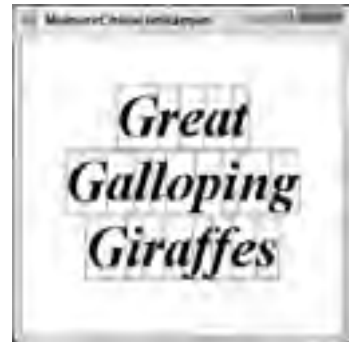
FIGURE 32-9: The Graphics object's MeasureCharacterRanges method shows where ranges of characters will be drawn in a string.
