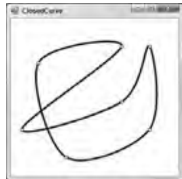
FIGURE 30-7: The DrawClosedCurve method draws a smooth curve connecting a series of points.
