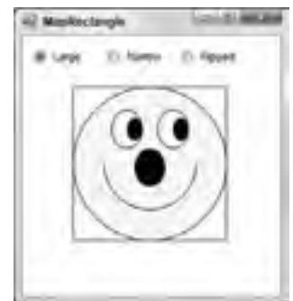
FIGURE 30-11: This program uses the MapRectangles subroutine to map a smiley face in world coordinates into a rectangle in device coordinates.
