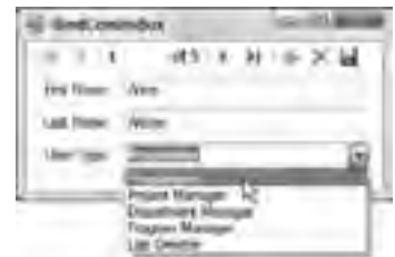
FIGURE 20-25: At runtime, the ComboBox displays the field bound to its DisplayMember property while updating the field bound to its SelectedValue property.
