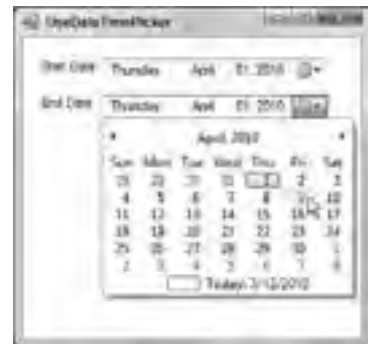
FIGURE G-3: The DateTimePicker control lets the user select a date and time.
