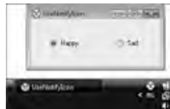
FIGURE G-6: The NotifyIcon component displays an icon in the system tray.
