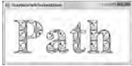
FIGURE 31-10: A program can use a Graphics object's FillPath and DrawPath methods to fill and draw a GraphicsPath object.
