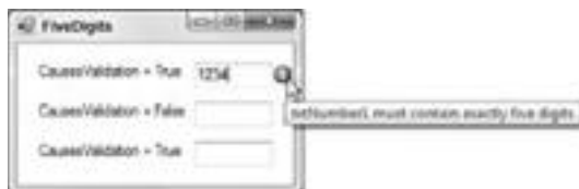
FIGURE 9-12: The Validating event fires when the focus moves to a control that has CausesValidation set to True.
