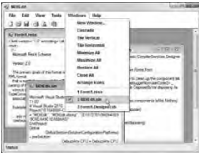
FIGURE 10-8: The MenuStrip's MdiWindowListItem property determines which menu item displays an MDI child list.
