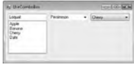
FIGURE G-2: The ComboBox provides three different styles: Simple , DropDown , and DropDownList .
