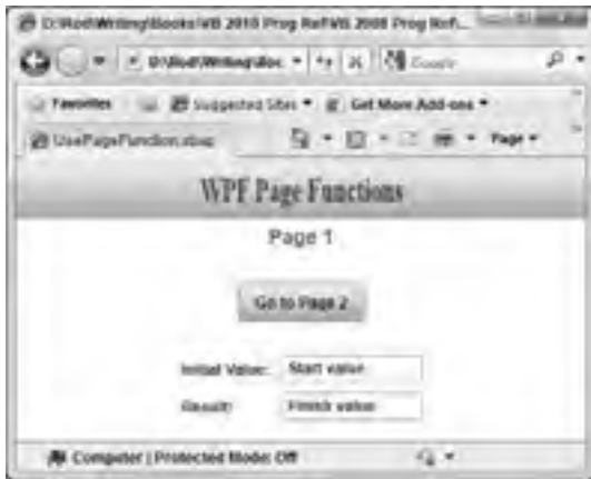
FIGURE 13-2: The PageFunction class simplifies passing parameters and return values to pages.
