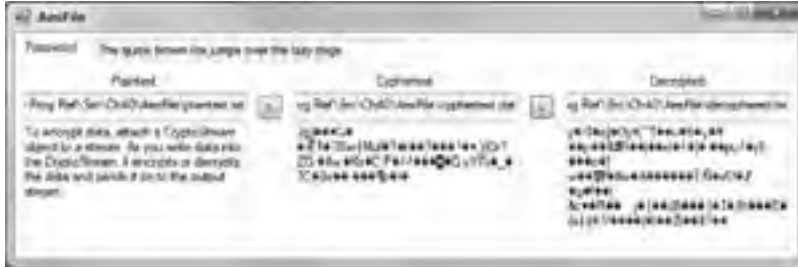
FIGURE 39-1: Changing even a single character in the password makes decryption produce an unintelligible result.
