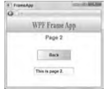
FIGURE 13-1: The Frame control provides navigation between Page objects.
