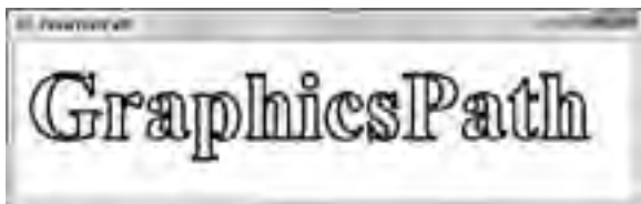
FIGURE 30-9: The DrawPath method draws the outline defined by a GraphicsPath object.
