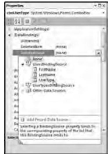
FIGURE 20-24: Set the BindingSource object's SelectedValue to the UsersBindingSource object's UserType field.
