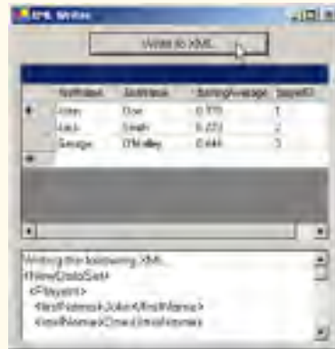
Fig. 19.30 XML representation of a DataSet written to a file (part 3 of 3).
