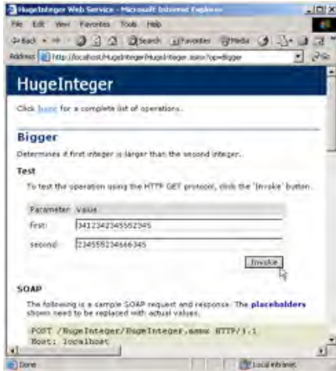
Fig. 21.3 Invoking a method of a Web service from a Web browser.
