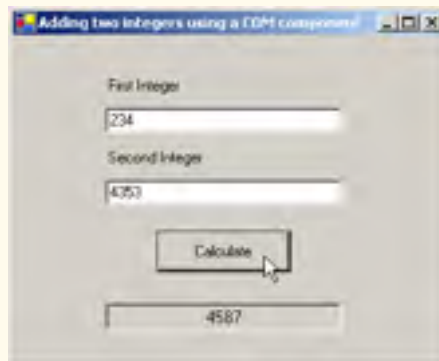
Fig. G.6 COM DLL component in Visual Basic.NET (part 2 of 2).
