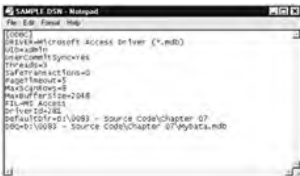
Figure 7-1: The SAMPLE.DSN file contains all of the settings required to use my database from within Visual C++.
