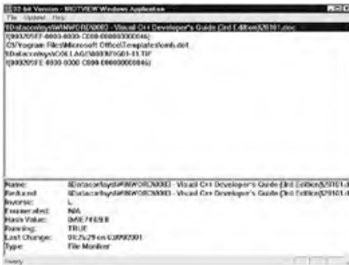
Figure 1-11: The main purpose of the IROTVIEW utility is to keep track of the OLE running object table.
