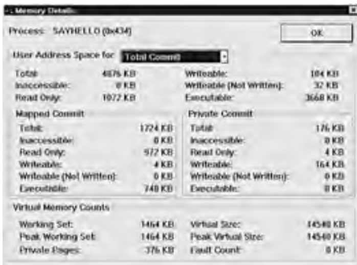
Figure 1-10: The Memory Details dialog box provides extremely detailed information about how a particular process is using memory.
