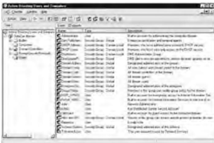
Figure 5-1: Use the Active Directory snap-in to view the entire network at a glance, although you can't manage some network details directly.
