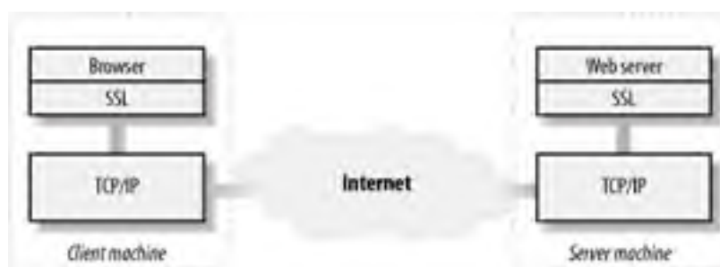
Figure 9-4. HTTP clients and servers, SSL, and the network layer that implements TCP/IP
