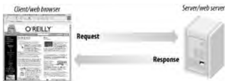
Figure 1-2. A web browser makes a request and the web server responds with the resource
