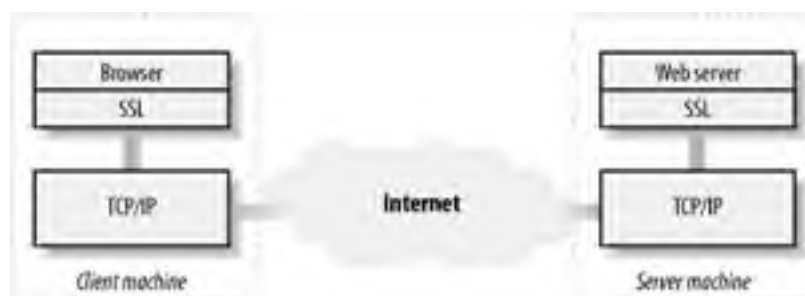
Figure 11-3. HTTP clients and servers, SSL, and the network layer that implements TCP/IP
