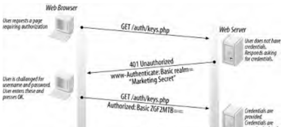
Figure 11-2. The sequence of HTTP requests and responses when an unauthorized page is requested
