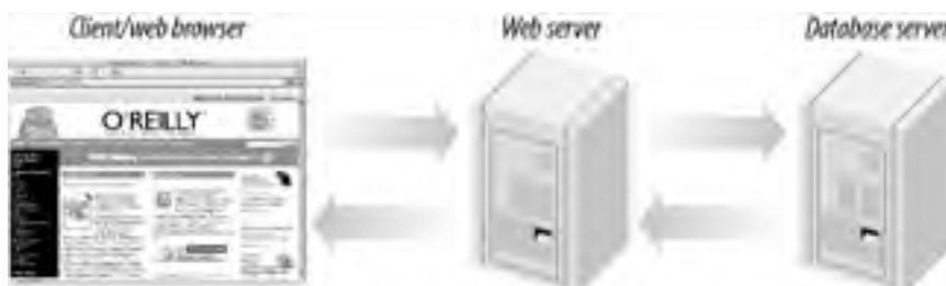
Figure 1-2. A three-tier architecture where a web browser requests a resource, and a response is generated from a database
