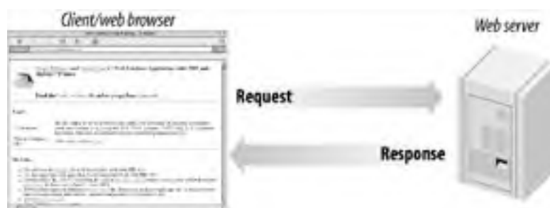
Figure 1-1. A two-tier architecture where a web browser makes a request and the web server responds
