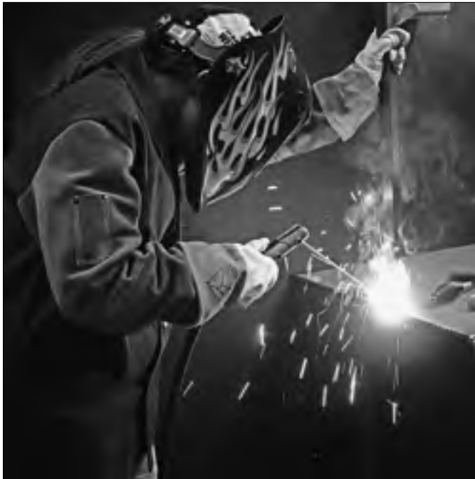
Figure 6-4: Welding an angle iron to your welding table.
