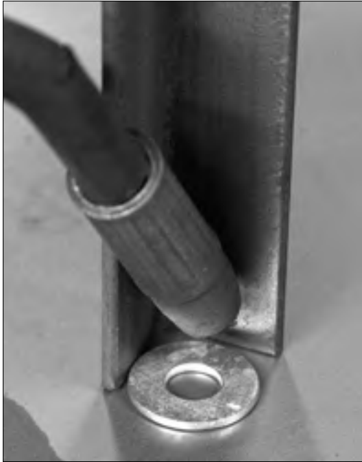
Figure 16-7: Position for welding the washers to the pieces of angle iron.
