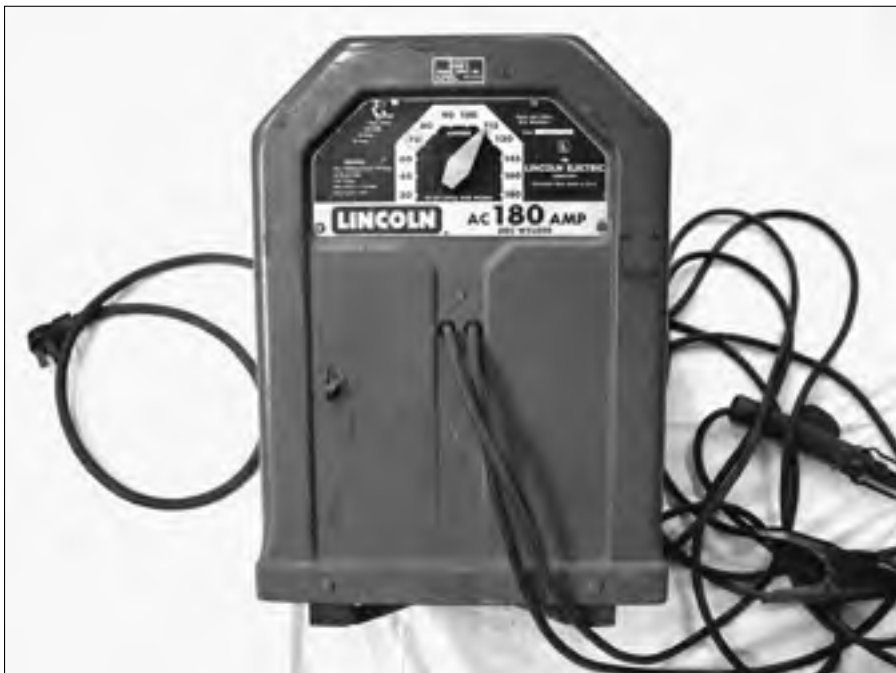
Figure 5-2: Transformer buzz box.
