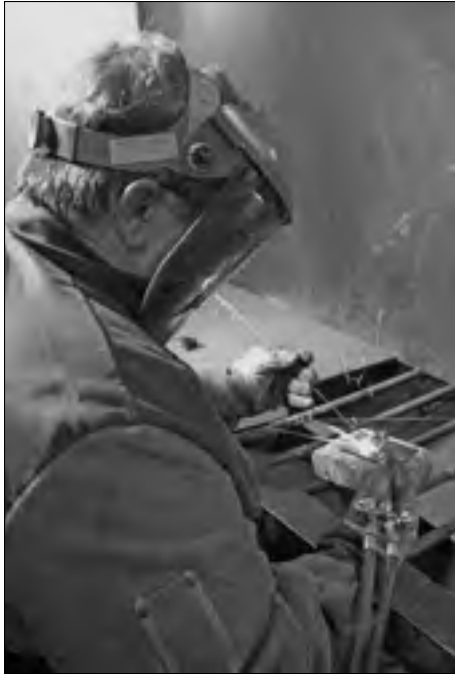
Figure 13-4: Fusion welding a butt joint with an oxyacetylene torch.
