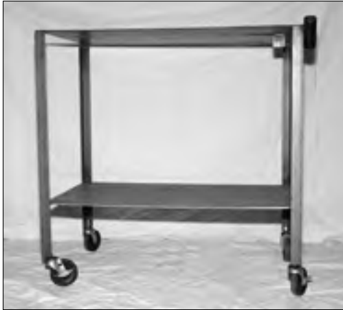
Figure 16-5: A completed portable welding table.
