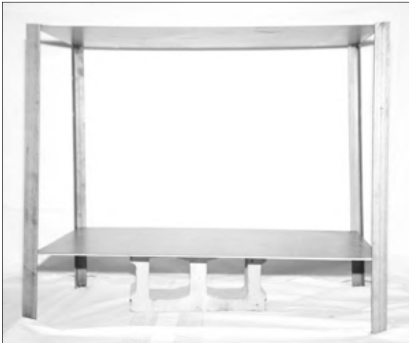
Figure 16-8: The partially constructed table lifted off the floor with spacers.
