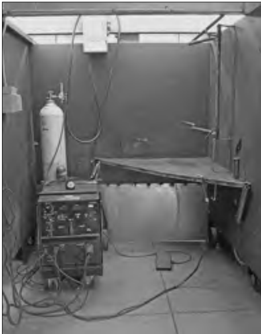
Figure 7-1: A tig welding setup.
