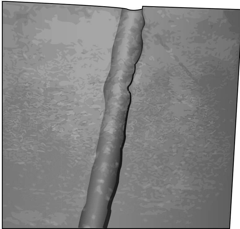
Figure 18-3: Example of a crack along a weld.
