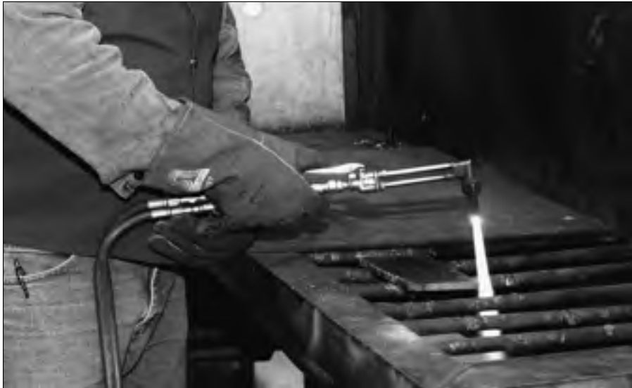
Figure 12-4: Operating an oxyfuel cutting torch.
