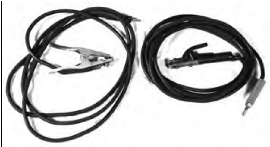
Figure 5-4: An electrode holder (left) appropriate for stick welding, along with ground clamp (right).
