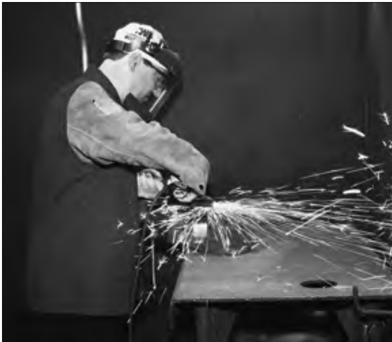
Figure 2-3: Cleaning steel with an angle grinder.
