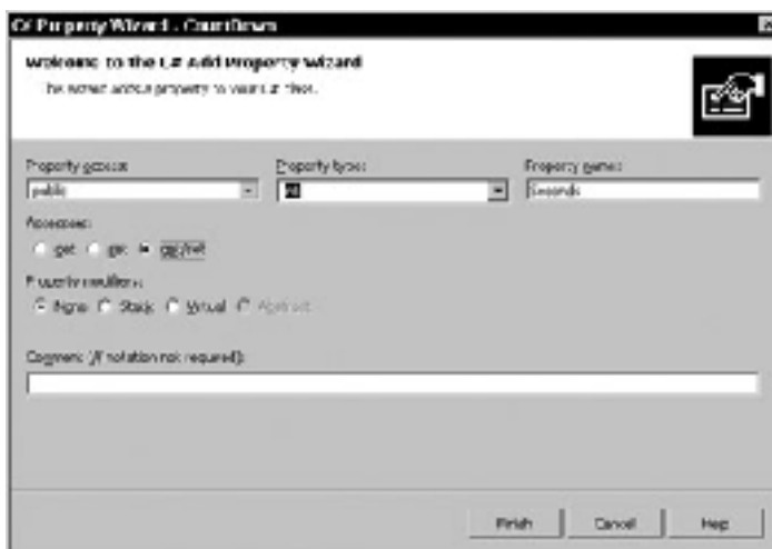
Figure 29-6: In the C# Property Wizard, name this property Seconds. Ensure that this property has public access and that the property type is set to Int.
