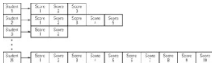
Figure 3-1: Jagged arrays let you define one array holding other arrays, each having a different number of elements.
