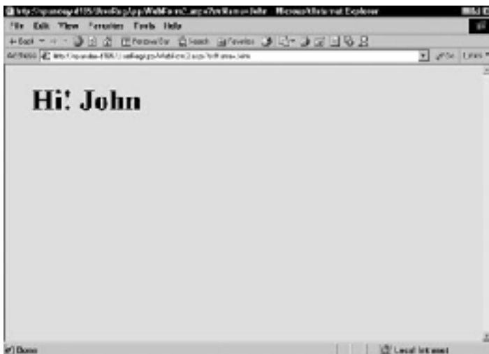
Figure 22-8: When a user is redirected to another page, the name of the user is passed in the query string.
