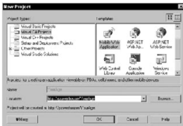
Figure 30-1: The new Mobile Web Application option was added when the Mobile Internet Toolkit was installed.
