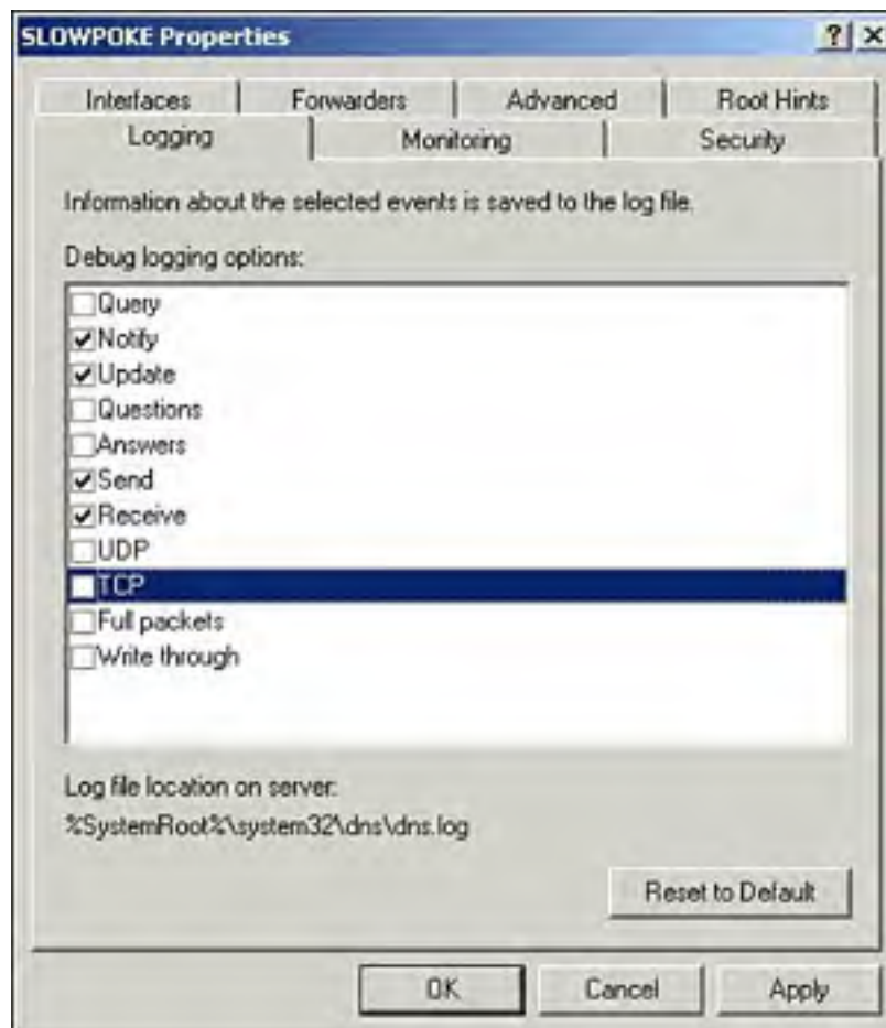
Figure 3.4. Logging is a useful troubleshooting tool when a DNS server is not responding as expected.
