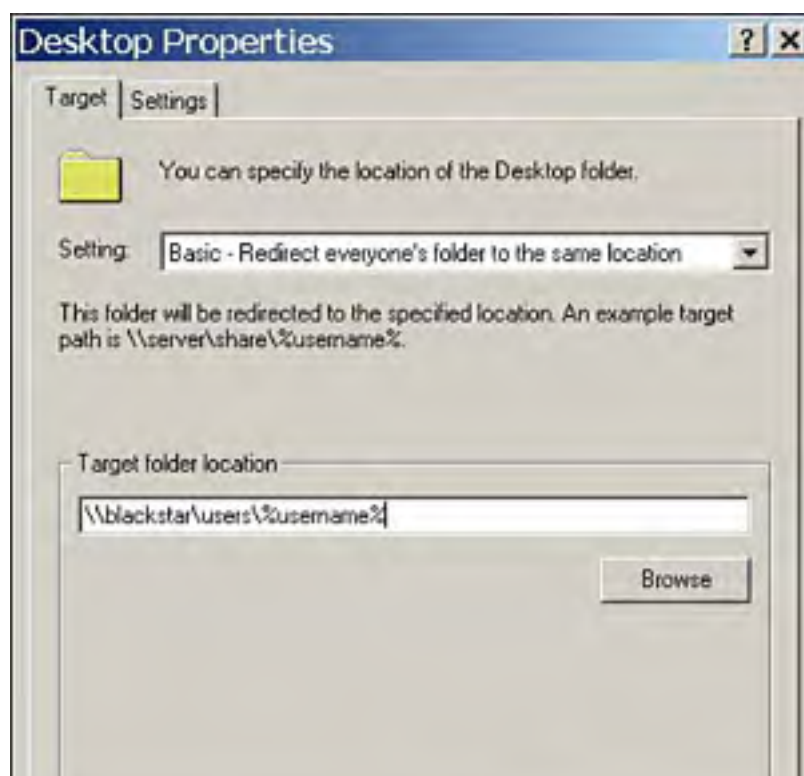
Figure 8.10. You configure Folder Redirection policies within the properties of a special folder.
