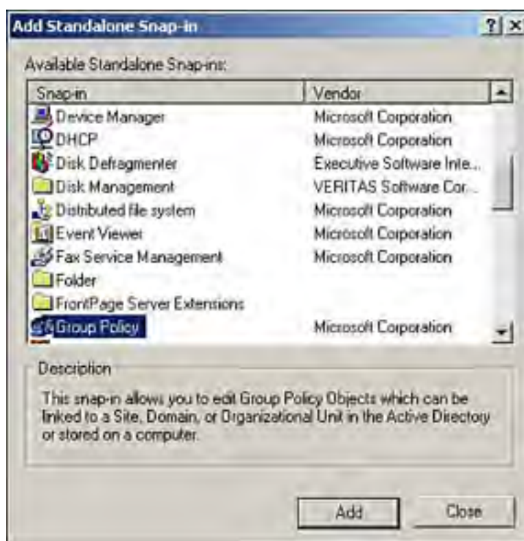
Figure 7.4. The list of snap-ins shows the available standalone snap-ins that can be added to the console.
