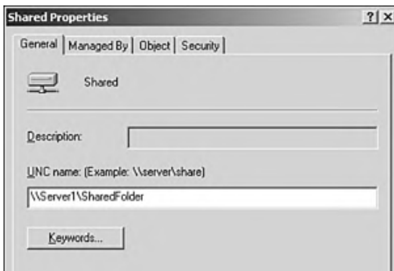
Figure 10.3. Adding search descriptions and keywords to a published folder with the AD.
