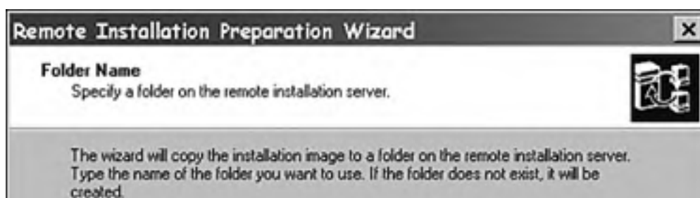
Figure 15.7. Supply a directory name on the RIS server for the Remote Installation Preparation Wizard to copy the image.
