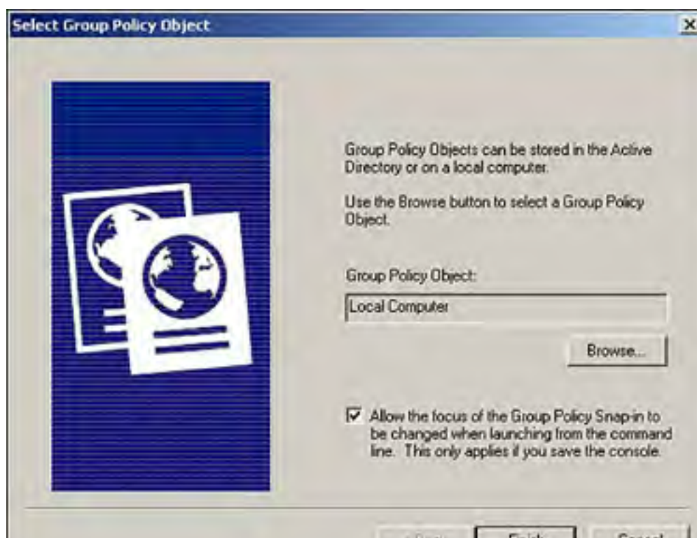
Figure 7.5. You must determine the focus of the Group Policy Editor when you add the snap-in to the console.
