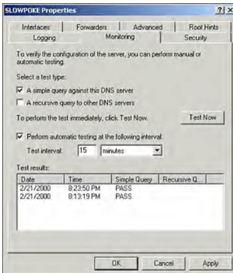
Figure 3.3. Windows 2000 enables an administrator to monitor the DNS service.
