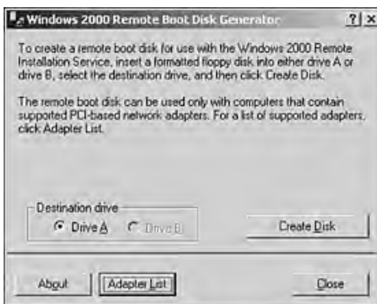
Figure 15.9. The RBF allows you to create a network-bootable disk for supported network adapters.
