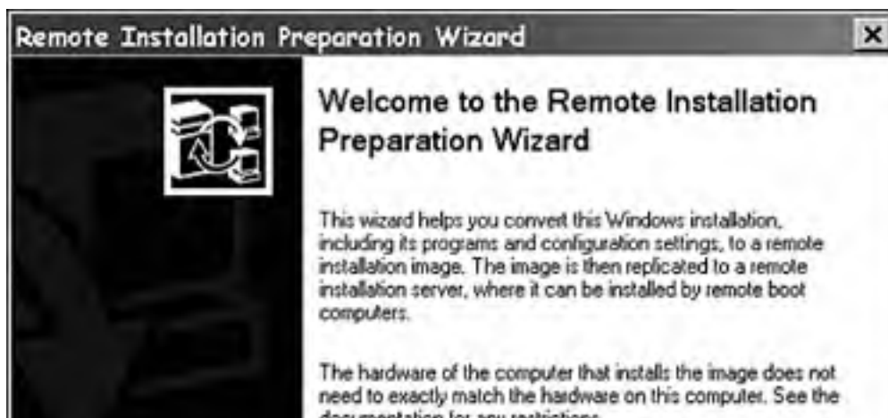
Figure 15.5. You start the Remote Installation Preparation Wizard by executing RIPrep.exe from a Windows 2000 Professional client computer.
