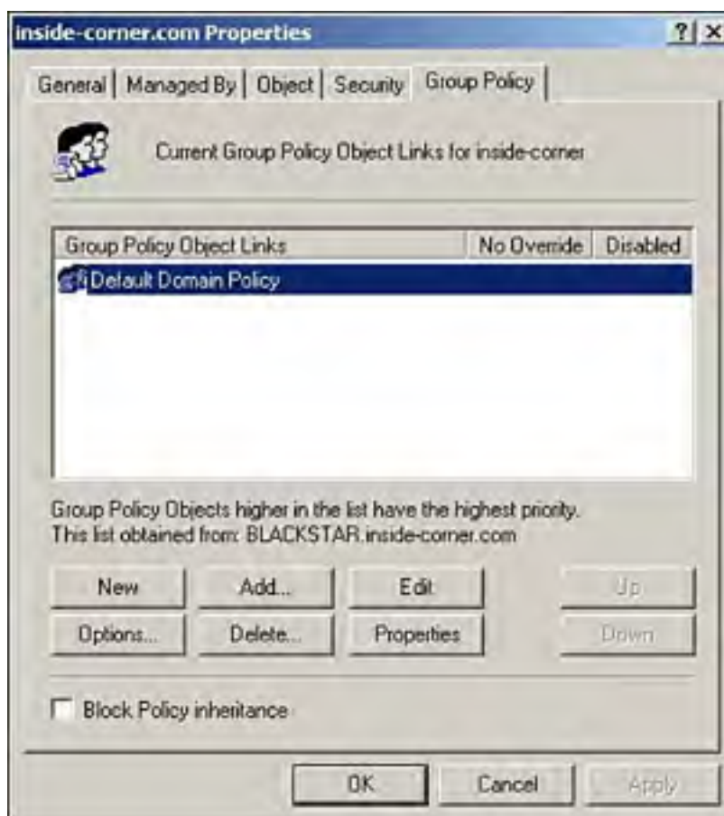
Figure 7.1. The Group Policy tab of a site, domain, or OU's properties dialog box supplies the options for creating, linking, and modifying GPOs.
