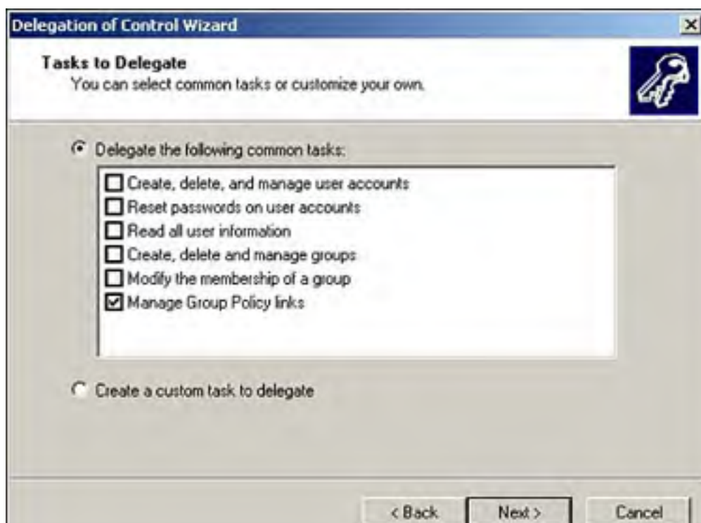
Figure 7.10. The Delegation of Control Wizard is used to delegate control of managing Group Policy links to users and groups.
