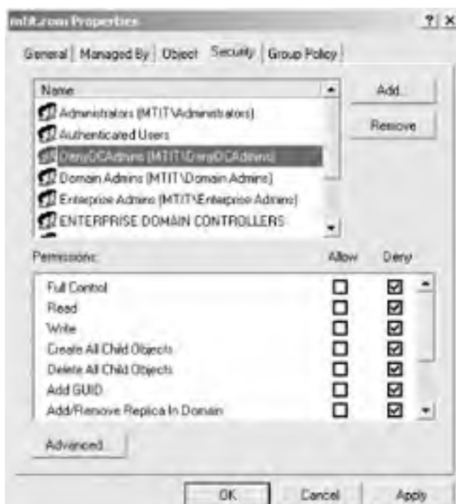
Figure 8-4. Denying Full Control permission for the DenyDCAdmins global group
