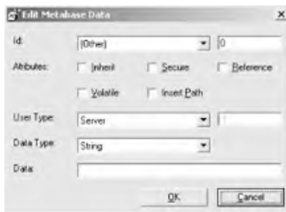
Figure 6-6. Adding a new property to the metabase based on its internal ID number
