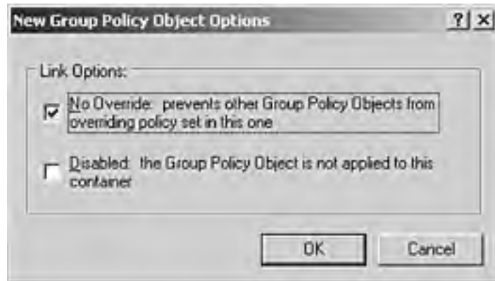
Figure 6.12. Configuring No Override is done through the Group Policy Object's Options button.
