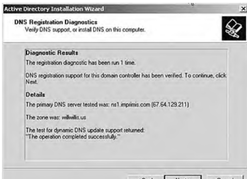
Figure 1.8. The AD Installation Wizard needs to determine the status of DNS prior to installation.
