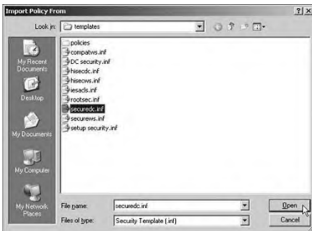
Figure 8.6. You can import Windows Server 2003 security templates into a Group Policy Object through the Computer Configuration container's Import Policy command.
