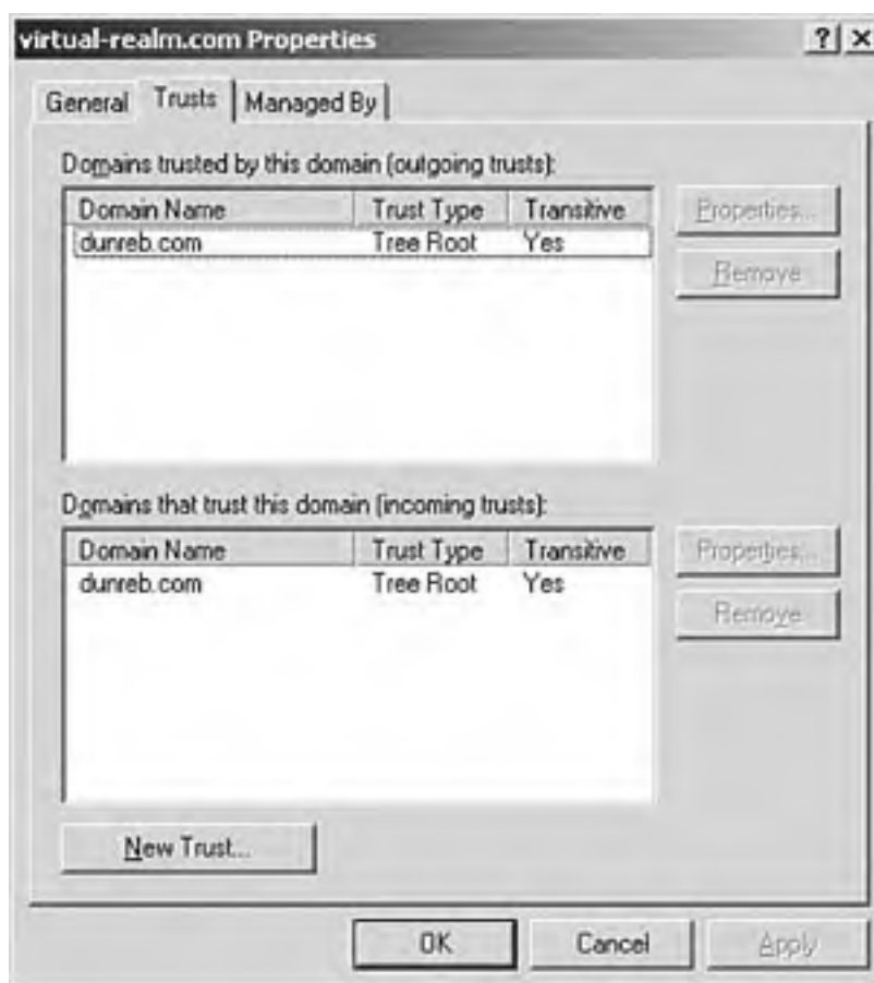
Figure 1.15. The Trusts tab of the domain properties is where you manually configure trust relationships.
