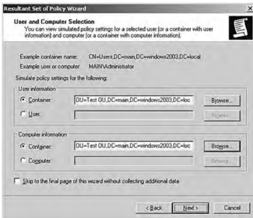
Figure 6.16. The User and Computer Selection screen of the Resultant Set of Policy Wizard.
