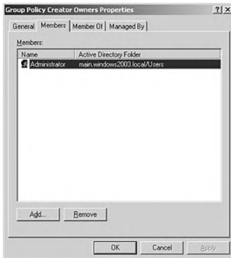
Figure 6.11. In order to create a GPO, a user or group must belong to the Group Policy Creator Owners group.
