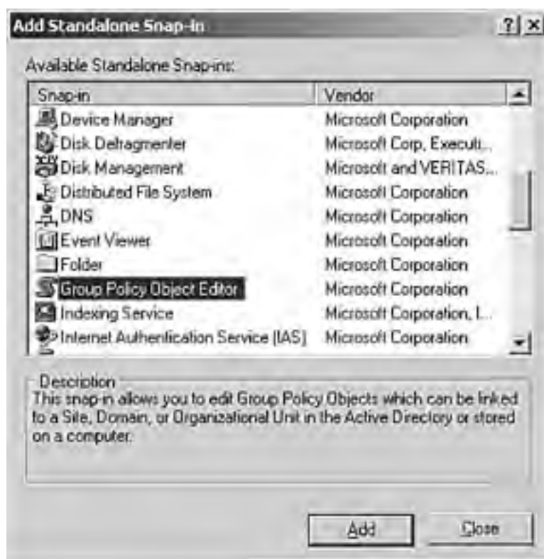
Figure 6.4. The list of snap-ins shows the available standalone snap-ins that can be added to the console.
