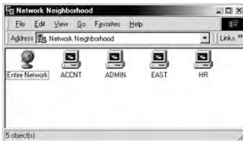
Figure 20-3. This workgroup has four computers. The Entire Network icon lets you drill down from the workgroup to the computers—but because you see the networked workgroup PCs immediately, there's little reason to do so.
