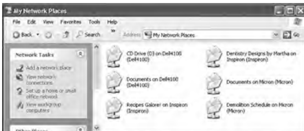
Figure 20-1. In Windows XP, all of the shared disks and folders show up automatically in the My Network Places window—including shared disks and folders on your own PC, which can be a bit confusing.
