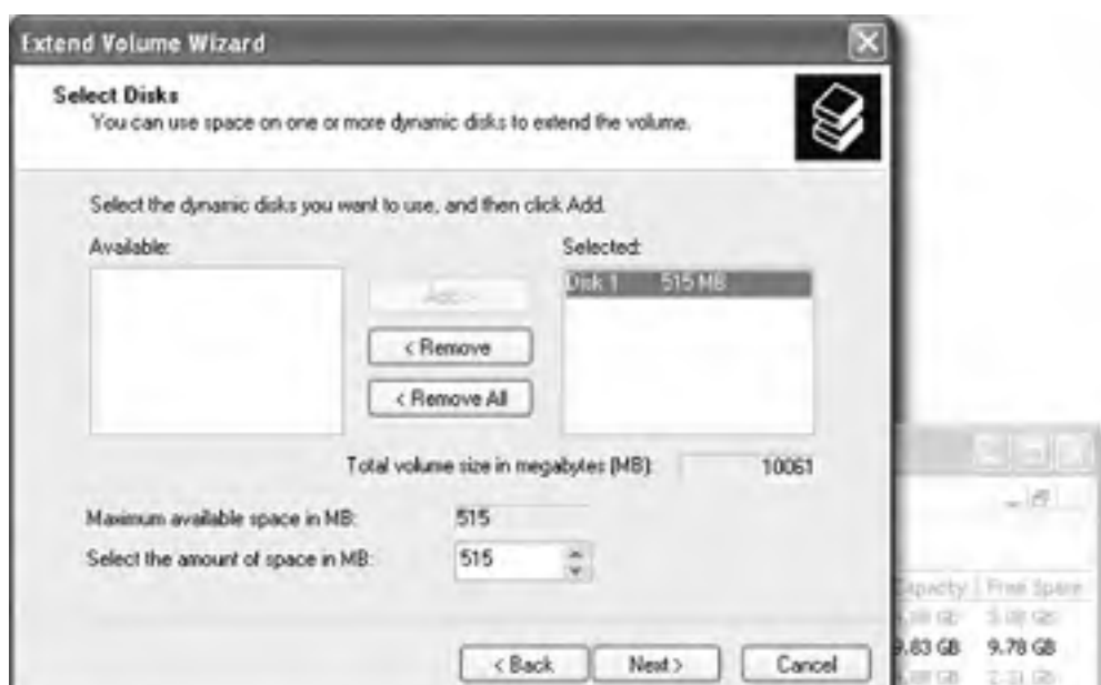
Figure 15-8. Top: When extending a volume to another disk, click its name in the Available column before adding it to the Selected column. Bottom: A dynamic volume extended to another disk appears in the Disk Management console with the same color header bar and the same drive letter. Note, too, that the volume list in the upper-right quadrant of this dialog box identifies this volume as "Spa..." (which, if you could see the whole word, would say "Spanned").
