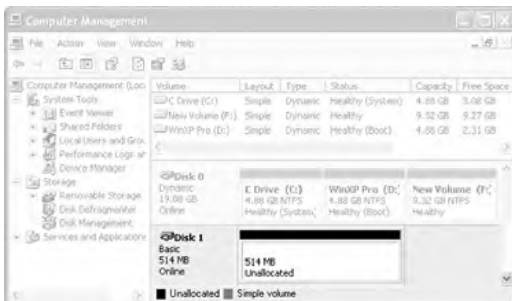
Figure 15-7. When you install a new hard drive in your computer, it appears in the Disk Management console as a large block of unallocated space. Of course, you quickly notice that the new drive is a basic drive; therefore, all you can do is create a basic partition on it.
