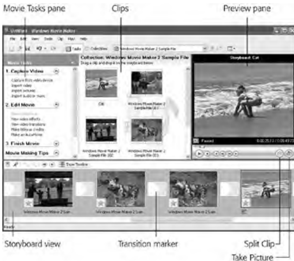
Figure 8-16. Windows Movie Maker 2 sports a new Movie Tasks pane that provides quick access to the most-used menu options. The other major working areas of the program are all identified here. You'll do most of your work in the Storyboard or Timeline view at the bottom of the screen.
