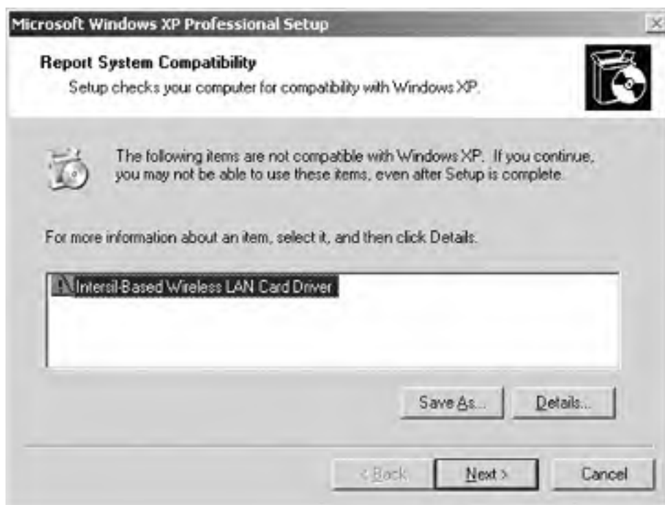
Figure A-3. This screen lists any programs and drivers that Microsoft considers incompatible with Windows XP Pro. You can save any information that shows up in this list to a file by clicking the Save As button.
