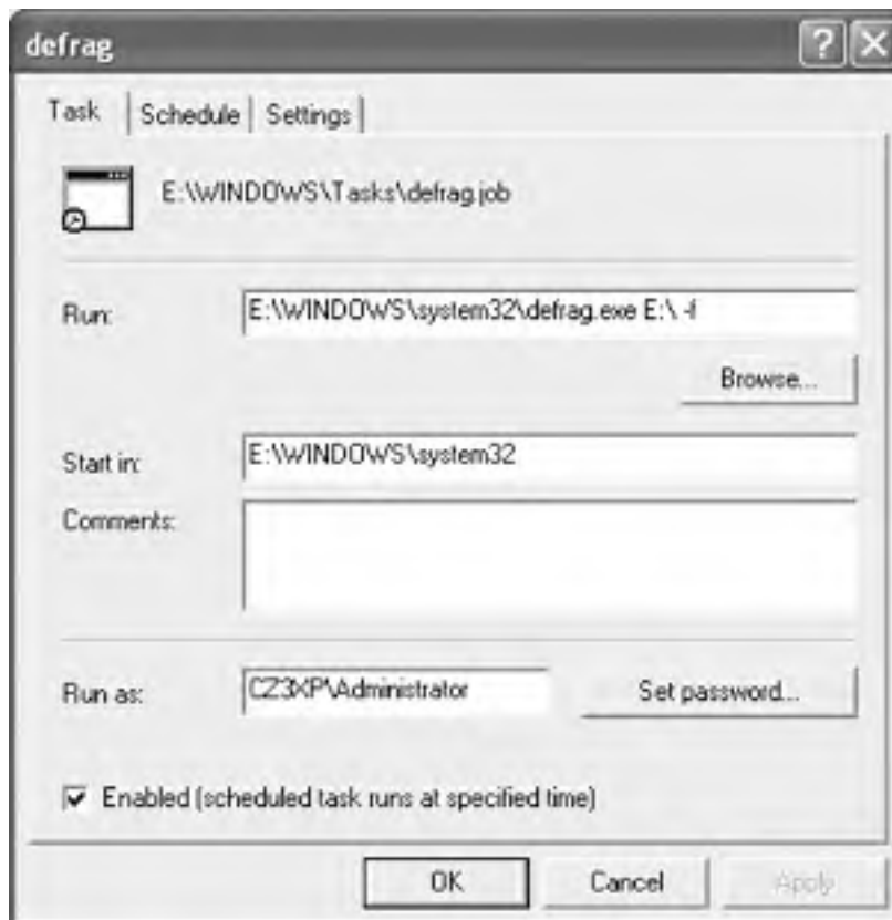
Figure 16-12. Disk Defragmenter is ready to roll. You've just told Disk Defragmenter to defrag the E: drive, and—thanks to the "-f" switch—to run whether it thinks you need it or not.
