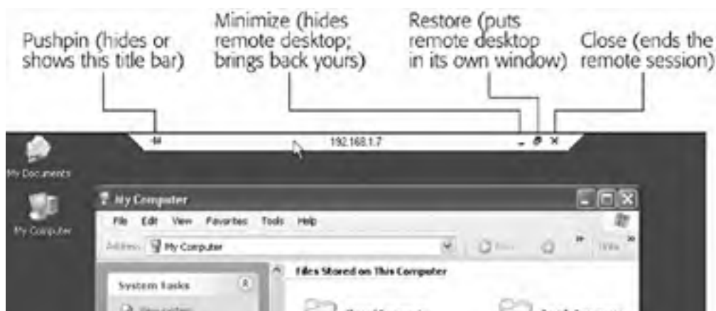
Figure 21-6. The strange little title bar at the top of your screen lets you minimize the distant computer's screen or turn it into a floating window. To hide this title bar, click the pushpin icon so that it turns completely horizontal. After a minute, it slides into the top of the screen, out of your way until you move the cursor to the top edge of the screen.
