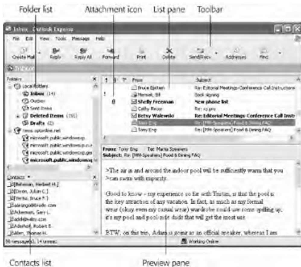
Figure 12-1. The four panes of Outlook Express. Click a folder in the upper-left pane to see its contents in the upper-right pane. When you click the name of a message in the upper-right pane, the message itself appears in the lower-right pane. Lower left: your list of MSN Messenger Service "buddies," as described in the previous chapter.
