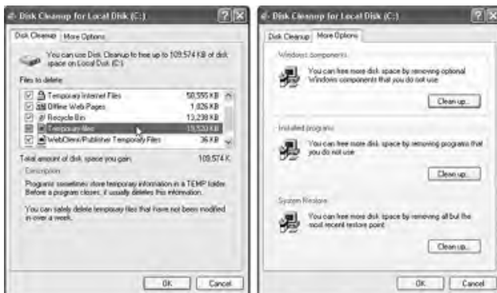
Figure 16-3. Left: Disk Cleanup announces how much free space you stand to gain. Click View Files to see the individual file icons in their native folders, for more selective deletion. Right: Links on the More Options tab lead to several uninstall functions, for quick removal of programs, Windows parts, and restore points.
