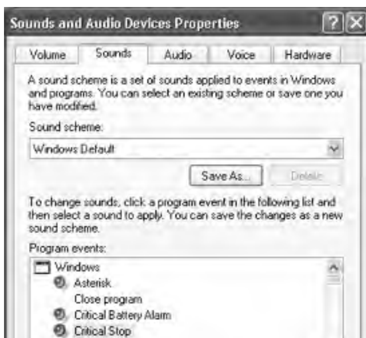
Figure 9-17. The Program Events list box presents every conceivable category in which a sound is played: Windows, NetMeeting, Windows Explorer, and so on. (The installers for some programs—America Online, for example—may add categories of their own.)
