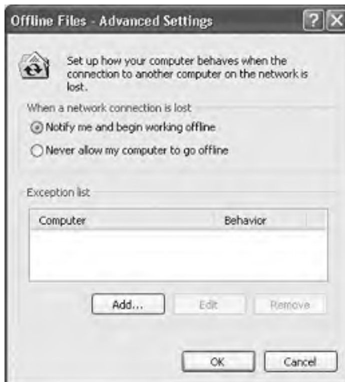
Figure 20-14. "Never allow my computer to go offline" doesn't actually prevent your computer from disconnecting from the network; it means that you'd rather stop working with offline files when the network connection is lost.
