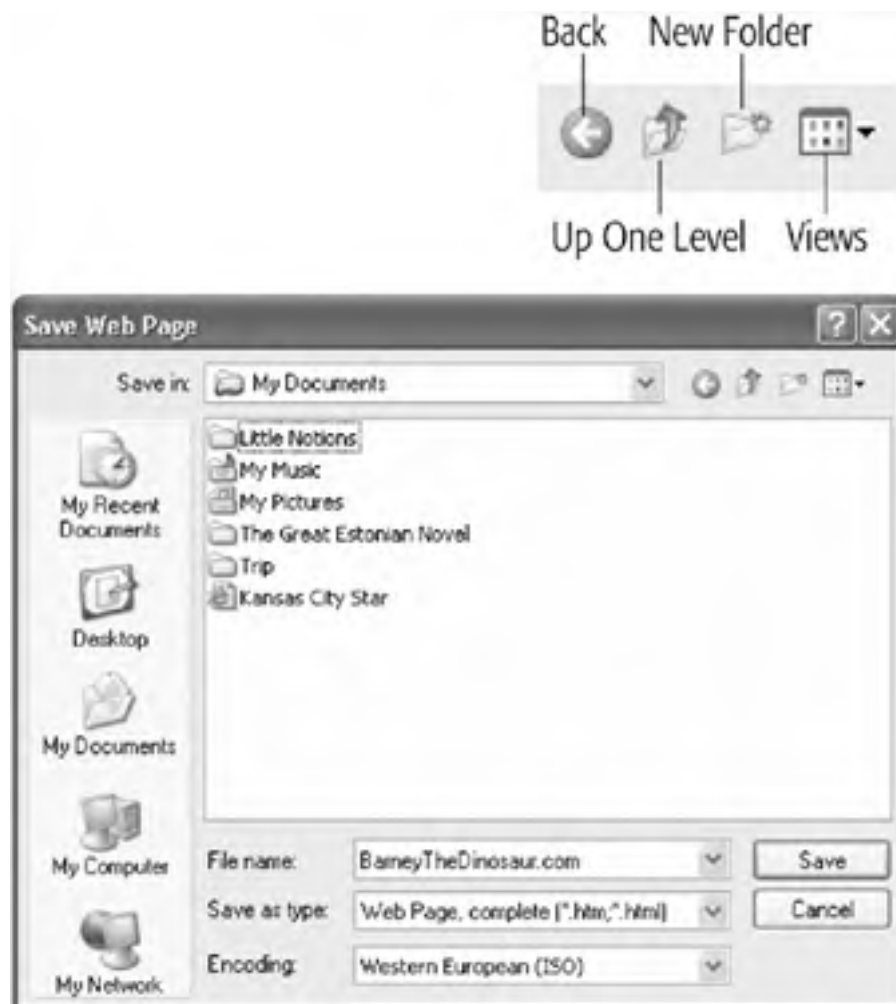
Figure 6-3. Top: These buttons vary by application, but the basics always help you navigate and view your files and folders. Bottom: The buttons at the left side of the Save As dialog box provide quick access to the folders where you're most likely to stash newly created documents: the My Documents folder, the desktop itself, and so on. But by using the "Save in:" drop-down list at the top of the screen, you can choose any folder you like.
