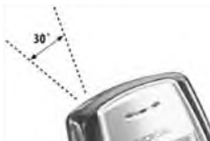
Figure 7-26. The 30 degree cone for peak power intensity of an infrared port
