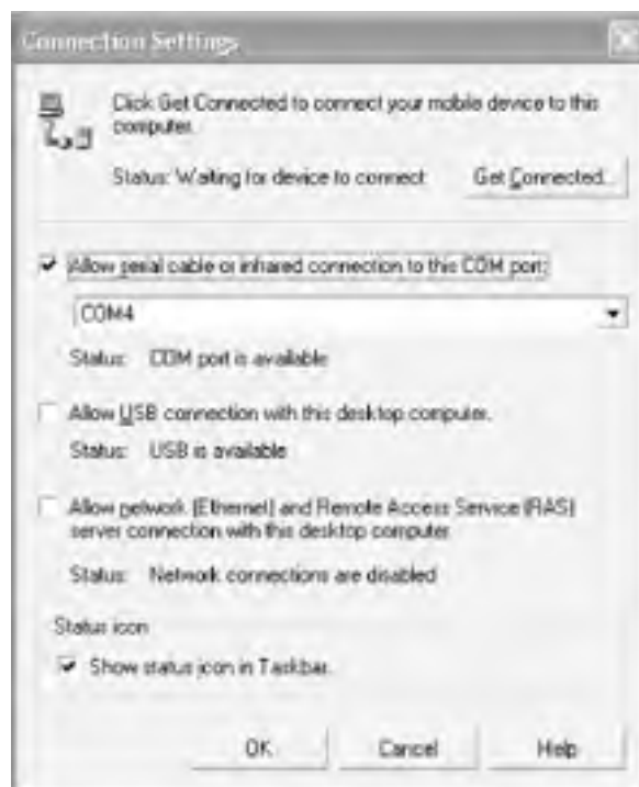
Figure 6-20. Setting a COM port for ActiveSync operation
