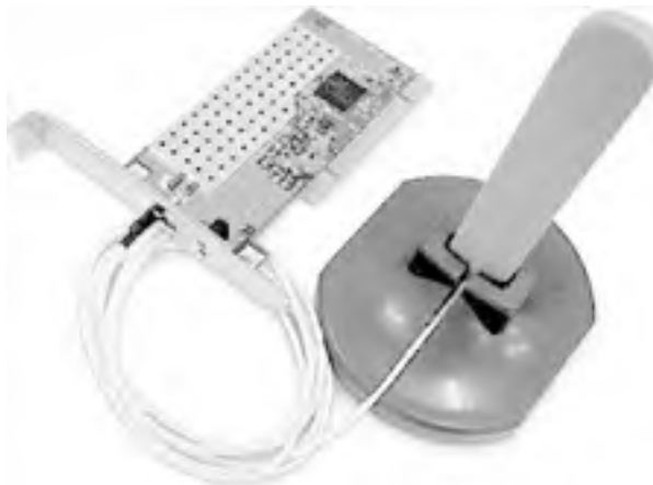
Figure 2-1. The D-Link AirPro DWL-AB520 Multimode Wireless PCI Adapter (802.11a and 802.11b)
