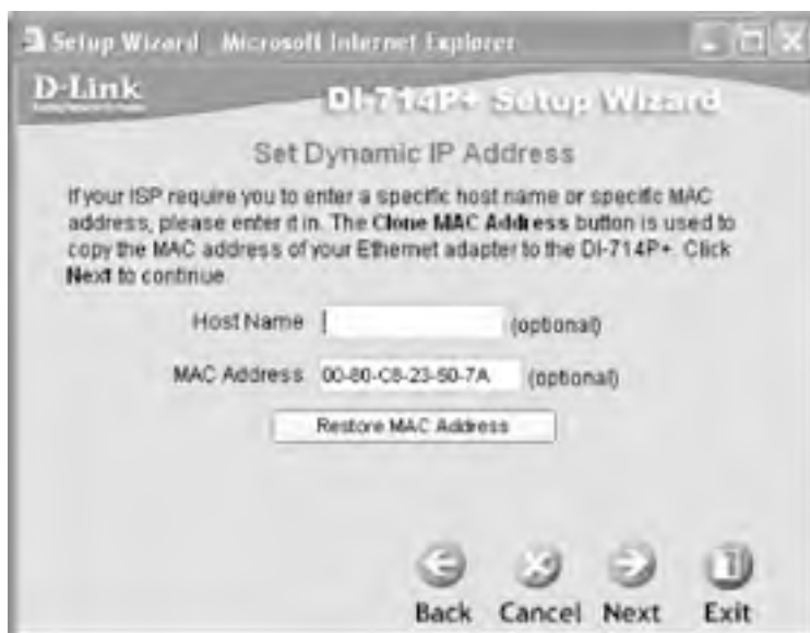
Figure 5-23. Setting the MAC address of the DI-714P+
