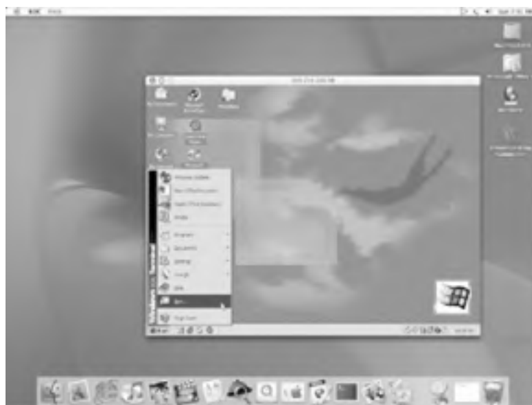
Figure 10-19. Using RDC (on a Mac) to connect to Windows 2000 Advanced Server
