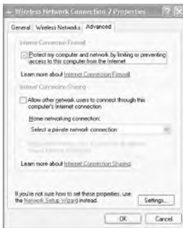
Figure 4-17. Enabling Windows XP's firewall
