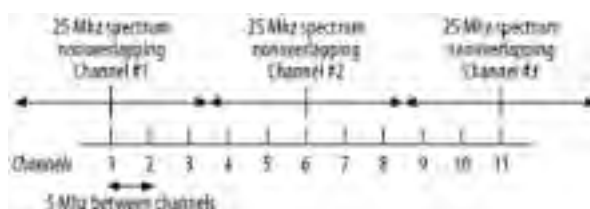
Figure 2-4. The nonoverlapping channels in 802.11b
