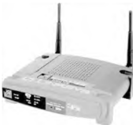
Figure 5-5. The Linksys WAP54G Wireless Access Point (802.11b and 802.11g) (photo courtesy of Linksys)
