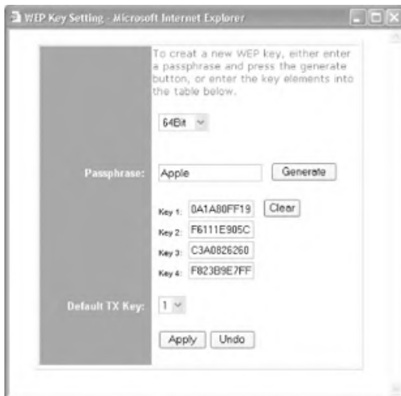
Figure 4-21 also shows the Linksys wireless access point using a passphrase to generate four WEP keys. You can also manually set any of the four keys as your WEP key without using a passphrase. After you set the keys, click Apply.
