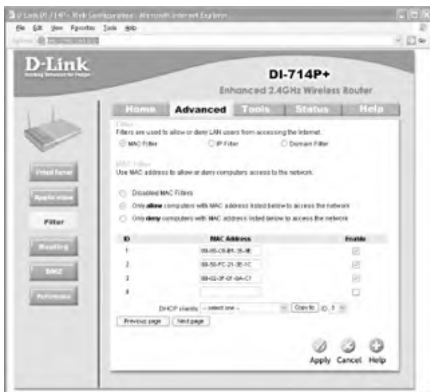
Figure 5-27. Specifying the MAC addresses for enabling wireless access (DI-714P+)
