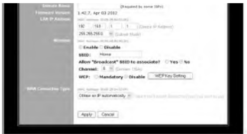
Figure 5-20 shows the web-based configuration utility of the DI-714P+. There are several tabs displayed horizontally: Home, Advanced, Tools, Status, and Help. Corresponding to each tab are various functions displayed vertically. For example, in the Home tab there are five functions: Wizard, Wireless, WAN, LAN, and DHCP.
