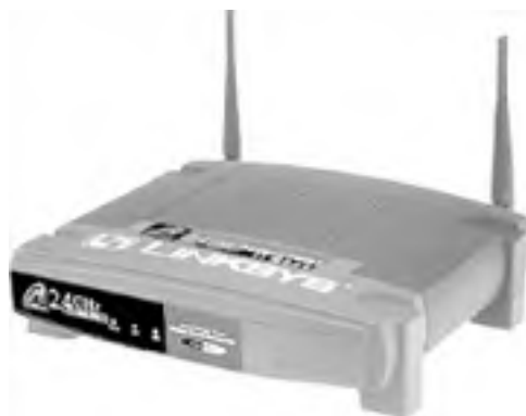
Figure 5-2. The Linksys WAP11 Wireless Access Point (802.11b) (photo courtesy of Linksys)
