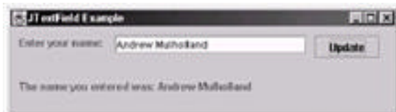
Figure 5: The label below the JTextField is updated to show the name the user entered.
