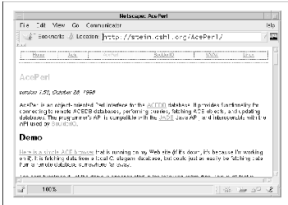
Figure 4.3. The navigation bar at the top of this page was generated dynamically by Apache::NavBar.
