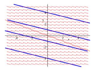
The *entire line* along the eigendirection  $\boldsymbol{\xi}^{(2)} = (2, -1)^T$  consists of equilibrium points. All other solutions diverge. The direction field changes across the line  $x_1 + 2x_2 = 0$ . Eliminating the exponential terms in the solution, the trajectories are given by
