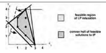
Here  $S = \{(1,2), (1,3), (2,1), (2,2), (2,3), (2,4), (3,0)\}$ . The optimal solution occurs at (1,3), with  $z_{IP} = \frac{1}{2}$ . The feasible region of the LP relaxation is also shown in Figure 3, with the optimal LP value  $z_{LP} = \frac{5}{4}$  attained at  $(0, \frac{5}{2})$ ; a cutting plane is shown as the dashed line. For this problem, *conv* (S) is defined by the following constraints:
