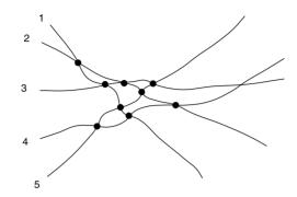
2. The following figure shows a standard way of representing a pseudoline arrangement as an *x*-monotone piecewise linear curve arrangement called a *wiring diagram*. The arrangement is the same as in the figure of Example 1.
