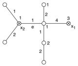
A 2-median of T is the set of vertices  $X_2 = \{x_1, x_2\}$ , with total transportation cost  $F(X_2) = 25$ . If  $x_1$  is kept fixed and t is an arbitrary point along edge e, then  $\{x_1, t\}$  also constitutes a 2-median of T. This is consistent with Fact 2, which only states that there is a p-median that is a subset of V, not that every p-median occurs in this way.
