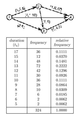
**2.** The paths from initial node 1 to terminal node 4 for the project in the figure of Example 1 are:  $Q_1 = [1, 2, 4], Q_2 = [1, 2, 3, 4], Q_3 = [1, 4], Q_4 = [1, 3, 4]$ . The following table lists the frequency and relative frequency that each path  $Q_i$ , or combination of paths, is a critical path.
