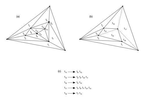
Algorithm 1 produces a hierarchy for planar subdivision. With minor modifications (for example, "triangles" become tetrahedrons), it can be used for subdivisions in  $\mathcal{R}^3$ . It can be proven that  $|T_{c \log_2 n}| = 1$  for some constant c, and that  $|\tau(t)|$  is a constant for every t.
