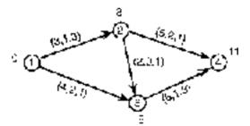
Each activity (arc) a is labeled with  $(u_a, \ell_a, k_a)$  where  $k_a$  is the marginal cost of reducing duration from the normal time  $u_a$ . Next to each node j is its earliest time of realization  $t_j(E)$  under normal activity durations. The following table summarizes the breakpoints of the resulting piecewise linear cost function.
