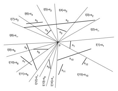
Algorithm 5, VisibilityMap, takes  $O(n \log_2 n)$  time and can be used for ray shooting among simple polygons. The visibility map consists of array  $\mathcal{I}$  and takes O(n) space. The problem is harder if the segments are allowed to intersect. Algorithm 6, RayShoot, takes  $O(\log_2 n)$  time.
