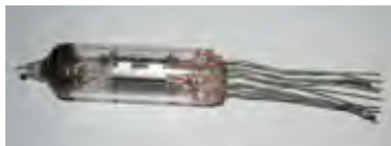
Subminiature CV4501 tube, 35 mm long x 10 mm diameter (excluding leads)
