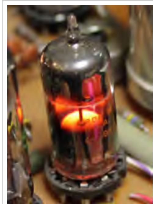
Voltage-regulator tube in operation. Low pressure gas within tube glows due to current flow.
