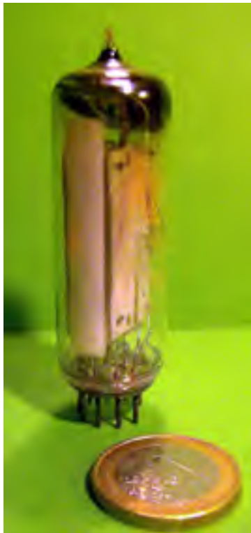
PM84 Miniature Magic Eye indicator tube, alongside a euro coin
