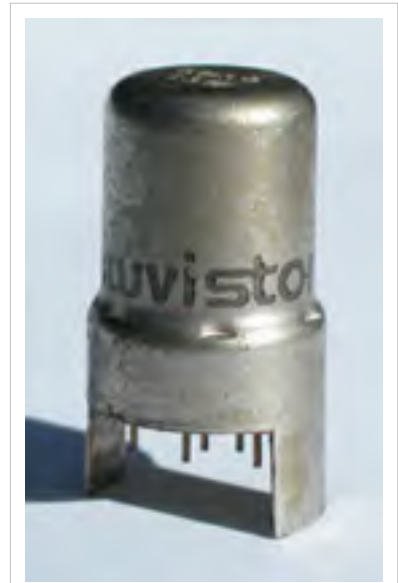
RCA 6DS4 "Nuvistor" triode, circa 20 mm high by 11 mm diameter
