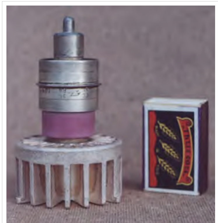
High power GS-9B triode transmitting tube with heat sink at bottom.
