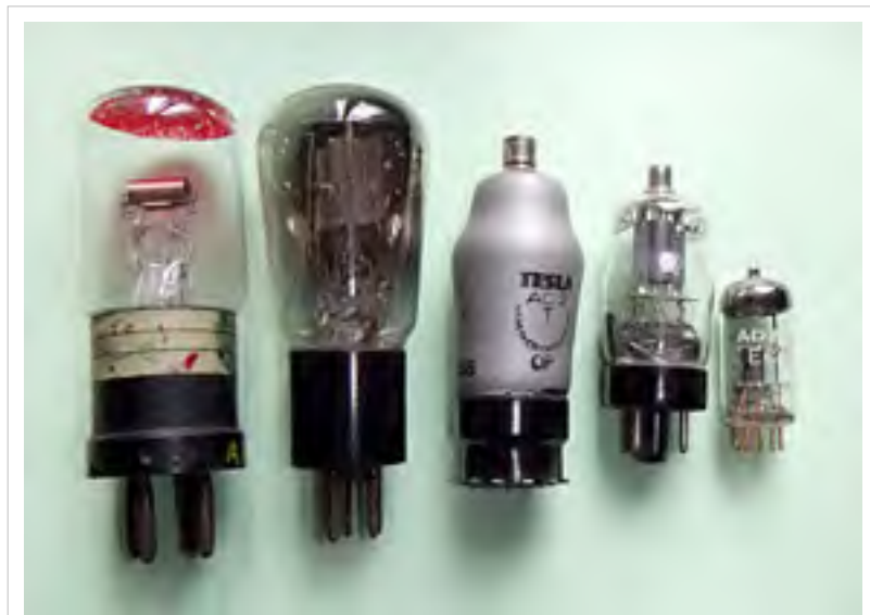
Triodes as they evolved over 40 years of tube manufacture, from the RE16 in 1918 to a 1960s era miniature tube.
