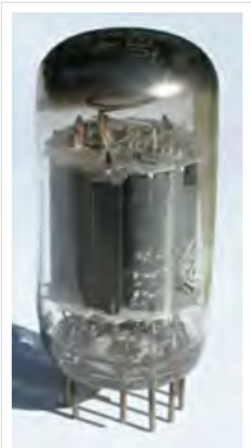
Compactron tube: 12AE10, dual pentode
