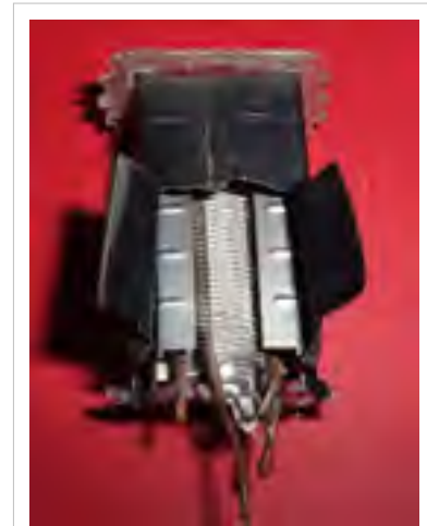
Vacuum tube with plate (anode) cut open revealing grid
