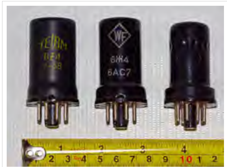
Metal cased tubes with "octal" bases
