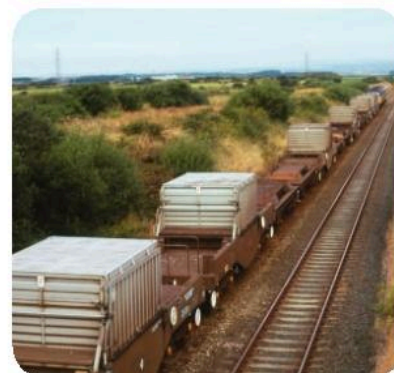
▲ The steel flasks on this train contain waste from a nuclear reactor
