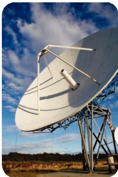
▲ This dish receives microwaves from a satellite.
