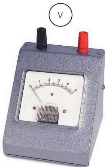
▲ Voltmeter and symbol. (For information about range and connection, see note under ammeter in previous spread.)
