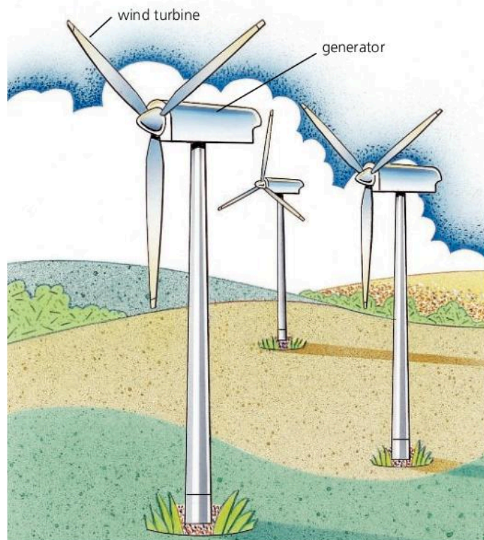
Wind farm This is a collection of aerogenerators – generators driven by giant wind turbines ('windmills').
