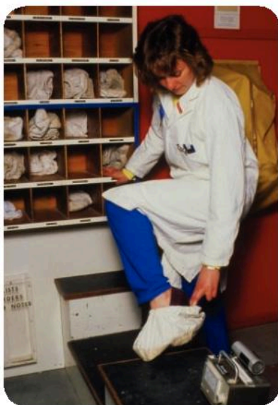
▲ This nuclear laboratory worker is about to use a GM tube and ratemeter to check for any traces of radioactive dust on her clothing
