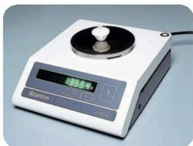
▲ A more modern type of balance. It detects the gravitational pull on the object on the pan, but gives its reading in units of mass.
