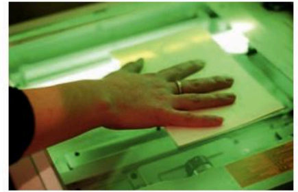
A bright light shines onto the original and is reflected onto the rotating drum
