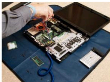
This electronic engineer is connected to the Earth through a wristband as he repairs a computer. Any static build-up in his body will discharge through the lead instead of damaging the delicate circuitry
