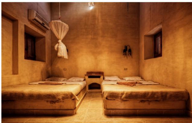
An air conditioning unit is used to cool the air in a hotel room. The cool air will fall directly onto the bed on the left
