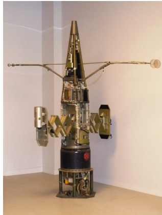
Figure 1.9. Dragon rocket (LPP collection). Several versions of this series were launched during the austral summer 1966–1967 from the Dumont d’Urville base by the CNES. The instruments are at the extremities of the arms that are deployed after launching. For a color version of this figure, see www.iste.co.uk/belmont/plasma.zip
