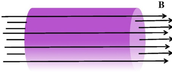
Figure 4.7. \theta -pinch configuration; balance is assured by a magnetic field B_z (black) along the plasma column (purple). For a color version of this figure, see www.iste.co.uk/belmont/plasma.zip
