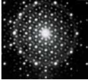
Figure 2.3.6: An electron diffraction pattern obtained from the Al_{78}Mn_{22} rapidly solidified alloy (Ref. [9]).
