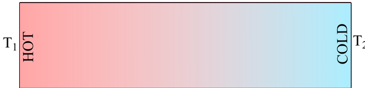
Figure 14.6.4: A bar of homogeneous material with a hot and a cold end (temperature gradient: this gradient of T points from the cold side to the hot side).
