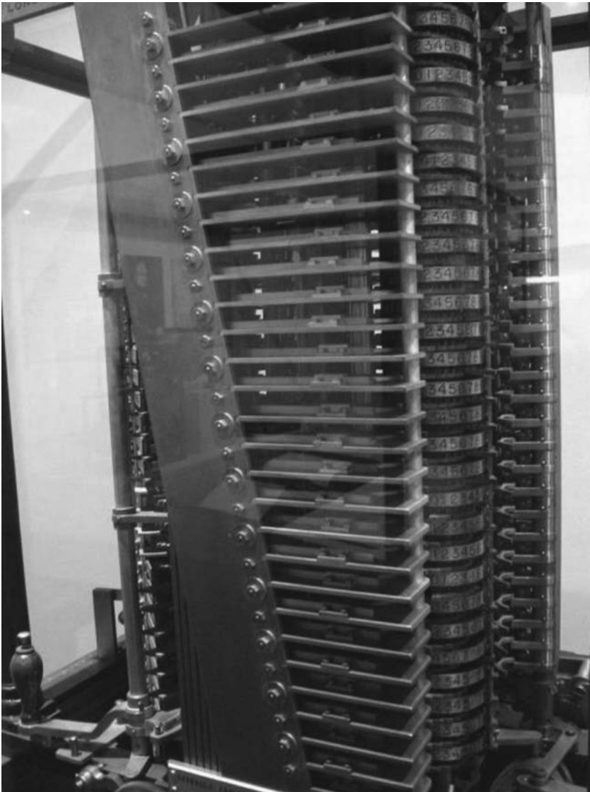
Figure 30.4. Henry Babbage's Analytical Engine Mill, built in 1910, on exhibit at the London Science Museum. (Wikimedia Creative Commons, author: Marcin Wichary, licensed under CC BY-SA 2.0.)
