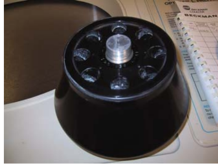
FIGURE 5.27 (upper) Modern ultracentrifuge; (middle) fixed angle rotor; (bottom) centrifuge remains after accident in which a rotor exploded while spinning.
