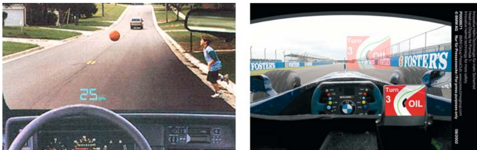
FIGURE 25.29 Head-up displays on a car windshield are holograms.
