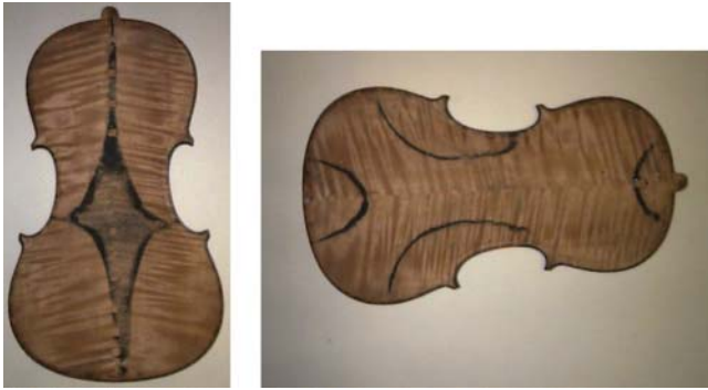
FIGURE 11.12 Examples of simple standing wave patterns on the back-plate of a violin. The dark lines, formed by black sand, represent nodal lines where the wood does not vibrate.
