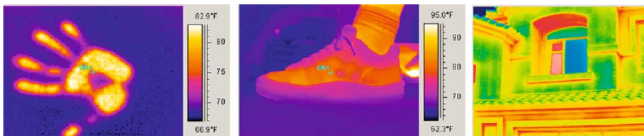
FIGURE 12.22 Examples of infrared imaging color-coded thermograms: (left) the imprint of a hand 5 min after touching a wall; (center) a shoe; (right) color-coded house showing heat leaks.
