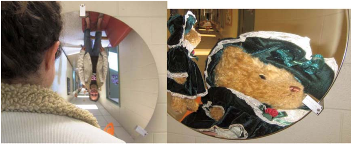
FIGURE 20.13 (left) Andrea's inverted image in a large concave mirror; (right) A Victorian bear and its image, with the bear located closer to the mirror than its focal point (see below) giving an enlarged upright image.
