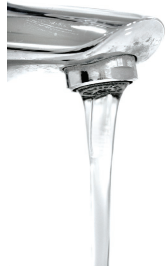
Figure 9.23 Demonstrating the continuity equation at a bathroom sink. Notice that the stream of water is narrower where the flow speed is faster. ©Michael Bodmann/Getty Images
