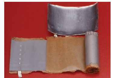
Figure 17.24 A disassembled capacitor, showing the foil conducting plates and the thin sheet of insulating material. ©Tom Pantages
