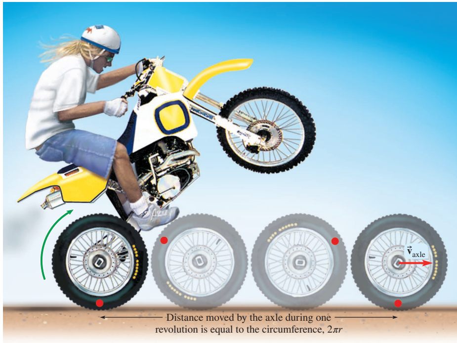
Figure 5.5 A wheel of radius r is rolling at constant speed v_{\text{axle}} without slipping. When the axle has moved a distance d equal to the circumference of the wheel ( 2\pi r ), the wheel has turned through one complete revolution ( \Delta\theta = 2\pi rad), as shown by the red dot on the tire. The elapsed time is the period T . Then v_{\text{axle}} = d/T = 2\pi r/T and |\omega| = \Delta\theta/T = 2\pi/T . We conclude that v_{\text{axle}} = |\omega|r for an object that rolls without slipping.
