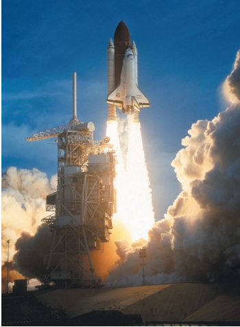
Figure 7.8 The Space Shuttle is propelled upward as hot gases are exhausted downward at high speeds from two solid-rocket boosters. The Shuttle program flew 135 missions during its 30 year existence (1981–2011). The five Shuttle orbiters were the first reusable spacecraft.
