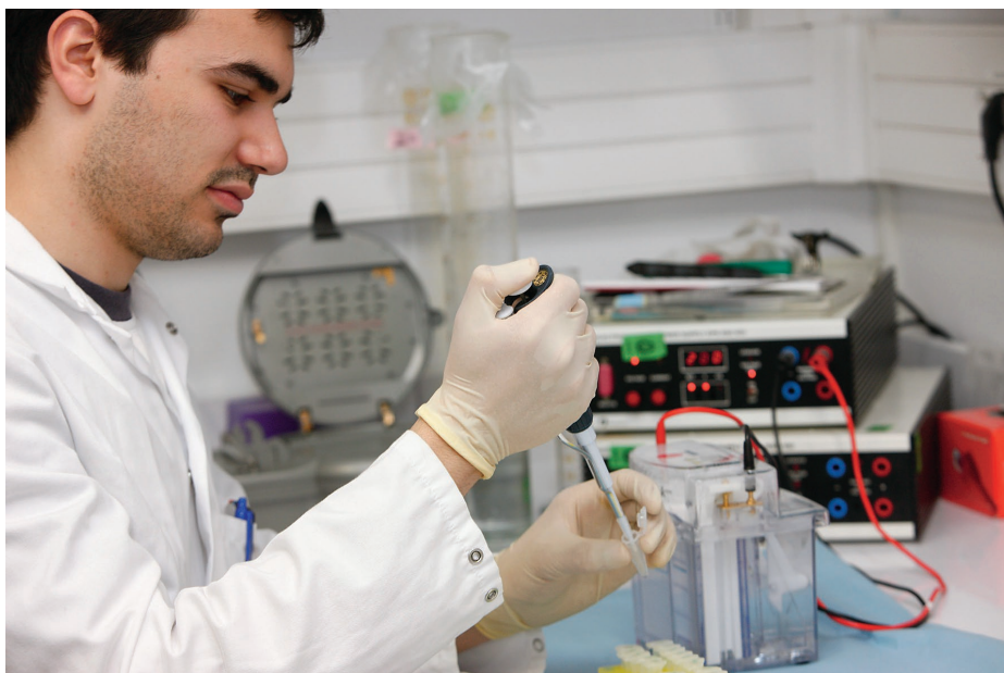
Figure 16.41 An apparatus used to perform gel electrophoresis. The molecules to be sorted are placed in wells in the gel. Then the power supply is turned on, subjecting the molecules to a large electric field and making them migrate through the gel.
