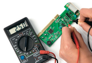
Figure 18.30 A digital multimeter being used to test a circuit board. A multimeter can function as an ammeter, as a voltmeter, or as an ohmmeter (to measure resistance). Most multimeters can measure both dc and ac currents and voltages. ©Oleksiy Maksymenko/Alamy
