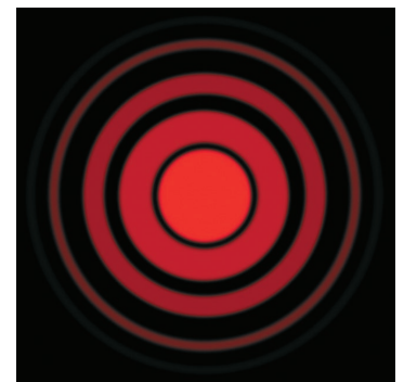
Figure 25.33 Diffraction pattern from a circular aperture on a distant screen. ©Tom Pantages
