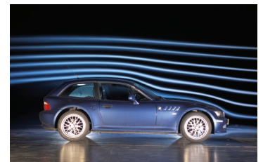
Figure 9.19 A wind tunnel shows the streamlines in the laminar flow of air past a car. ©culture-images GmbH/Alamy
