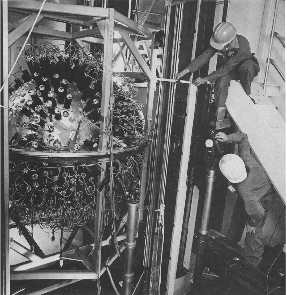
Figure 35.8. The crystal ball detector at SLAC. Numerous photomultiplier tubes bristle from the surface of the spherical container. They are monitoring the sodium iodide crystals mounted in the interior which detect the photons originating from the interaction point. (Photo courtesy SLAC.)
