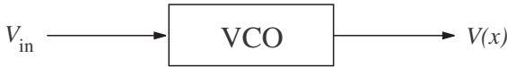
Figure 1.1. A voltage-controlled oscillator. The controlling voltage V_{\text{in}} is applied to the circuit, and the output has a fixed periodic waveform ( V ) whose phase x is modulated by V_{\text{in}} .
