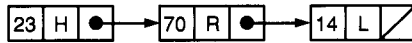
Figure 5.4 Sparse array represented as a linked list. Each list element contains Index, Value, and Next fields; each Value field stores a character.
