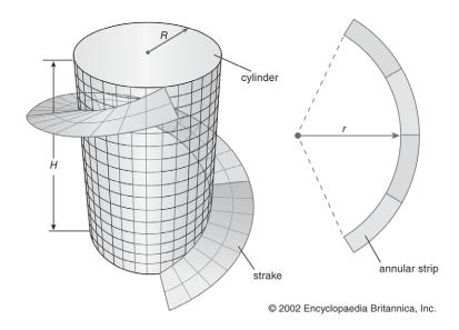
An annular strip (the region between two concentric circles) can be cut and bent into a helical strake that follows approximately the contour of a cylinder. Techniques of differential geometry are employed to find the dimensions of the annular strip that will best match the required curvature of the strake.
