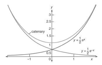
Any nonelastic, uniform cable held at its ends will droop in the shape of a catenary. As shown here, the catenary is asymptotic in the negative and positive directions to graphs of, respectively, exponential decay  $(y = e^-x/2)$  and exponential growth (y = ex/2). Copyright Encyclopaedia Britannica; rendering for this edition by Rosen Educational Services
