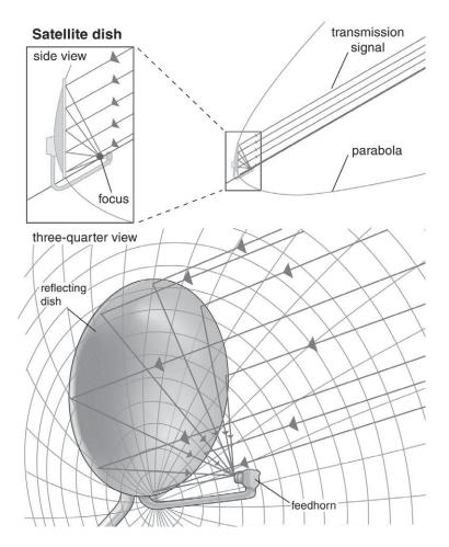
Satellite dishes are often shaped like portions of a paraboloid (a parabola rotated about its central axis) in order to focus transmission signals onto the pickup receiver, or feedhorn. Typically, the section of the paraboloid used is offset from the centre so that the feedhorn and its support do not unduly block signals to the reflecting dish. Copyright Encyclopaedia Britannica; rendering for this edition by Rosen Educational Services
