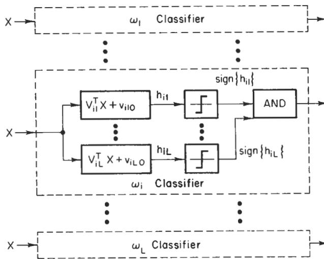
Fig. 4-13 Implementation of a piecewise linear classifier.
