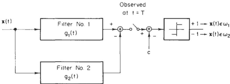
Fig. 4-3 Block diagram of a matched filter classifier.
