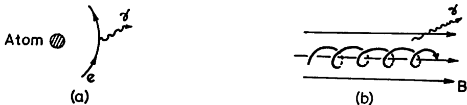
FIG. V.2 (a) Bremsstrahlung (braking radiation): electromagnetic energy emitted by a rapidly moving charged particle when it is slowed down by an electric field; (b) Synchrotron radiation : radiation emitted by relativistic charged particles moving in circular or helical orbits in a magnetic field.
