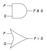
An AND gate turns its output current on only when both of its sources of input current are on; otherwise, its output current remains off. And, as you may have guessed, an OR gate outputs current when either of its input sources are on; otherwise, its output remains off.
