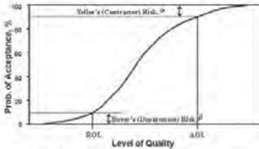
Figure 3 - Typical Operating Characteristic (OC) Curve for an Accept/Reject Acceptance
