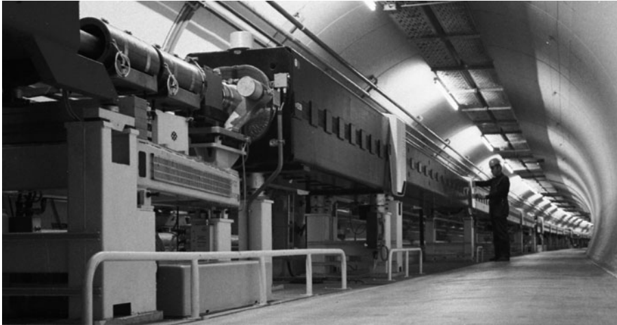
The tunnel of the proton-antiproton collider at CERN. The same bending magnets and focusing can be used for protons or antiprotons moving in opposite directions. The rectangular box in the foreground is a focusing magnet; the next four boxes are bending magnets. [CERN.]
