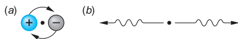
FIGURE 2-11 (a) A positron orbits with an electron about their common center of mass, shown by the dot between them. (b) After a short time, typically of the order of 10^{-10} s for the case shown here, the two annihilate, producing two photons. The orbiting electron-positron pair, suggestive of a miniature hydrogen atom, is called positronium .
