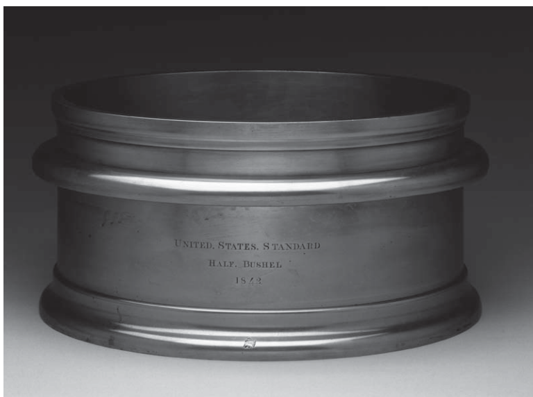
A brass measure representing the size of half of the U.S. bushel. SSPL/ Getty Images
