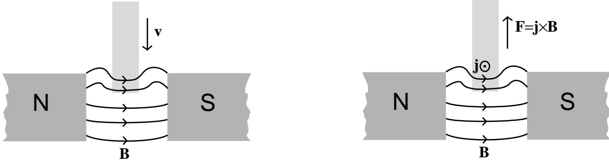
Fig. 18.1: The two key physical effects occurring in MHD. (a) A moving conductor modifies the magnetic field by appearing to drag the field lines with it. When the conductivity is infinite, the field lines appear to be frozen into the moving conductor. (b) When electric current, flowing in the conductor, crosses magnetic field lines there will be a Lorentz force, which will accelerate the fluid.
