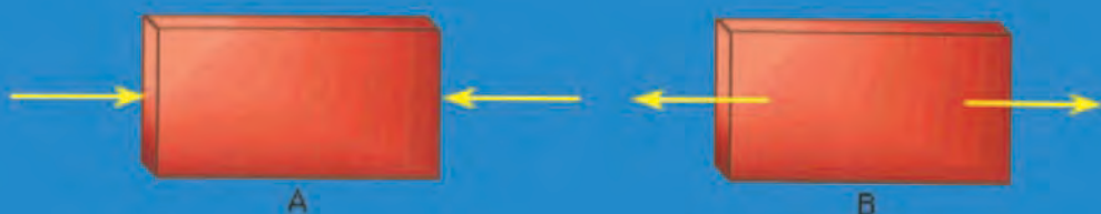
(A) Compression produced by equal and opposite forces. (B) Tension produced by equal and opposite forces. Copyright Encyclopædia Britannica; rendering for this edition by Rosen Educational Services
