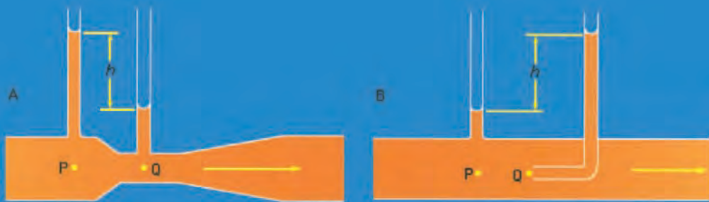
Schematic representation of (A) a venturi tube and of (B) a pitot tube. Copyright Encyclopædia Britannica; rendering for this edition by Rosen Educational Services
