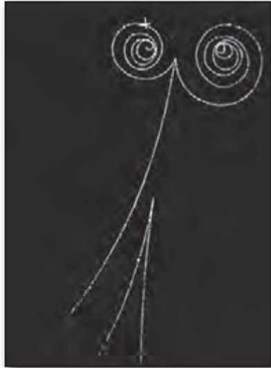
Electrons and positrons produced simultaneously from individual gamma rays curl in opposite directions in the magnetic field of a bubble chamber. Here the gamma ray has lost some energy to an atomic electron, which leaves the long track, curling left. The gamma rays do not leave tracks in the chamber, because they have no electric charge. Courtesy of the Lawrence Berkeley Laboratory
