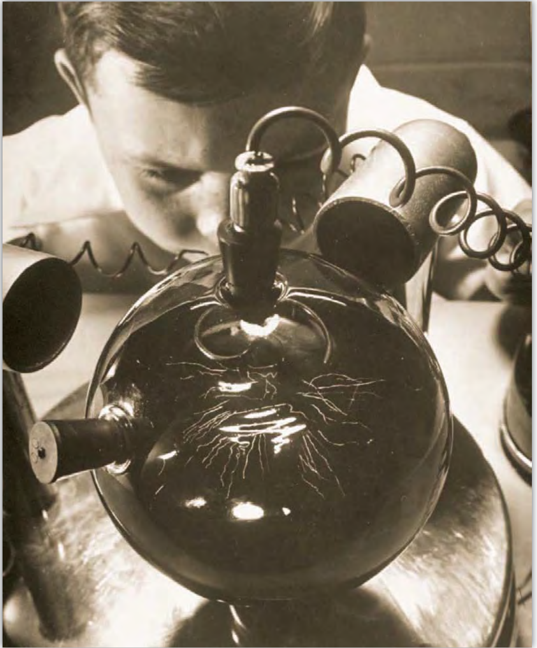
The Wilson cloud chamber detects the path of ionizing particles, but Patrick Blackett began to develop it into an automatic instrument to investigate cosmic radiation. Bernard Hoffman/Time & Life Pictures/Getty Images
