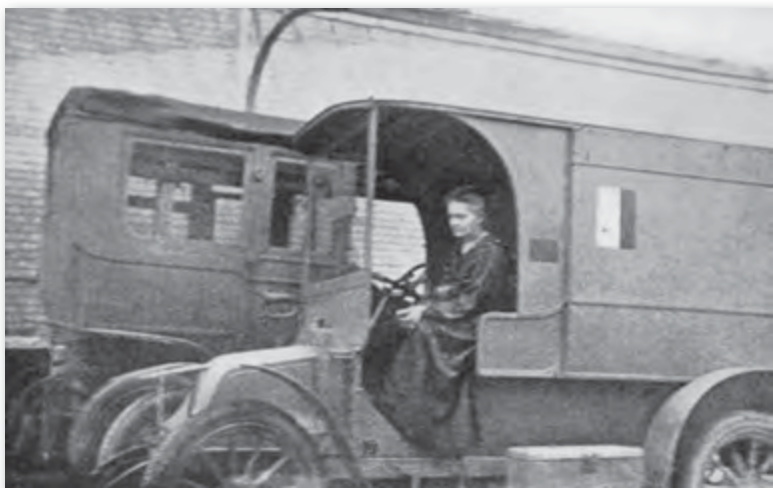
Marie Curie driving a Renault automobile converted into a mobile radiological unit, 1914. Curie used these vehicles, which became known as petites Curies, to bring X-ray equipment to wounded soldiers at the front during World War I. © Photos.com/Jupiterimages
