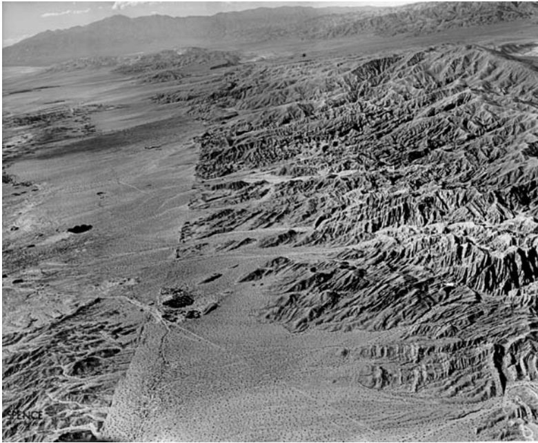
FIGURE 14.2 Mismatch of geological features across a branch of the San Andreas fault near Indio, California. Photograph by Spence Air Photos.
