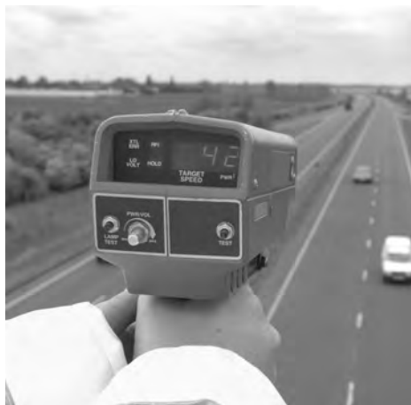
Radar guns used by police to monitor traffic speeds work by taking advantage of the Doppler Effect.
