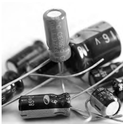
The modern capacitor is an updated version of the Leyden jar, consisting of two conductors and an insulator.
