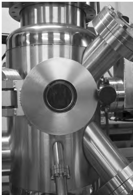
Modern vacuum chambers like this one are used in laboratories to study atoms, molecules, nuclei, and electrons. Otto von Guericke invented the vacuum pump in 1690 to help him study electricity in a vacuum, and since then vacuums have been used to study such things as cathode rays and electrons.
