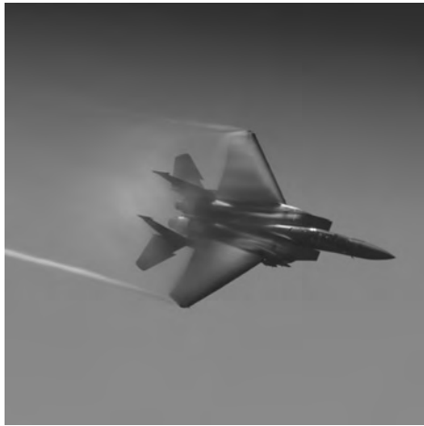
Supersonic planes, such as this F-15 fighter jet, can go beyond Mach 1. When they do, they generate a “sonic boom” caused by sound waves piling up and creating a shock wave.
