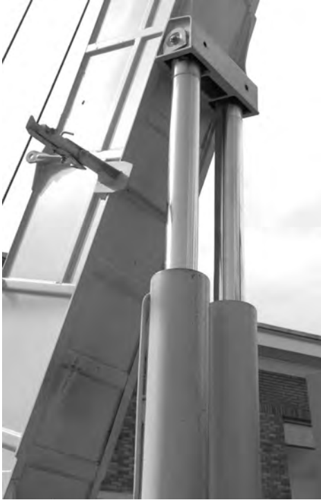
This heavy crane boom uses hydraulics to lift the boom.
