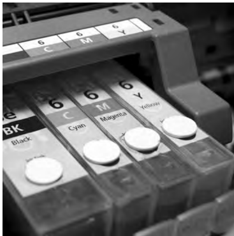
Color inkjet printers use black, along with yellow, cyan, and magenta, because the colored pigments do not cover the full spectrum. Therefore, they cannot produce a dark black but only a muddy dark brown.
