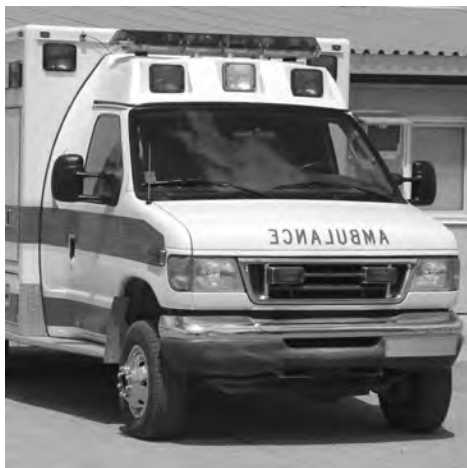
The word "AMBULANCE" is printed backwards on these emergency vehicles so that drivers will see the word correctly in their rearview mirrors.
