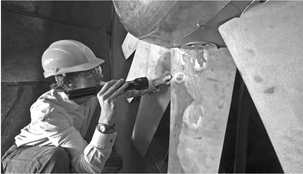
An engineer checks the fan in a wind tunnel. Smoke introduced into wind tunnels makes streamlines visible, which in turn help with the analysis of the efficiency of airfoils and automobiles.
