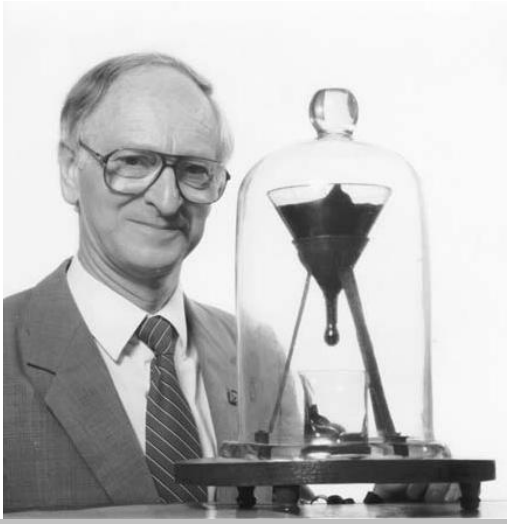
pitch drop experiment Professor John Mainstone alongside the world's longest-running experiment. John Mainstone, University of Queensland
