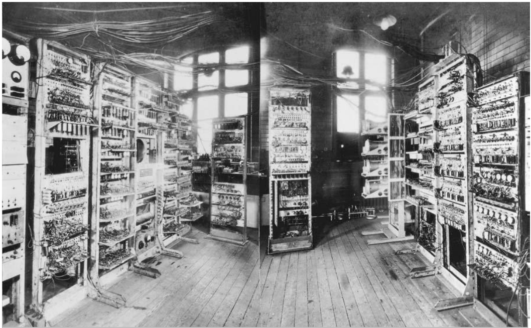
Babbage, Charles The realization of Babbage's dream: the Manchester Mark 1 computer at Manchester University, England, in 1948. This was the first computer that could store both data and programs electronically. Ferranti Electronics Ltd.
